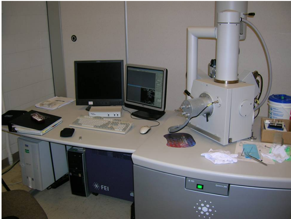
Figure 25. FEI FP 2011/11 Quanta 200 HV scanning electron microscope.
