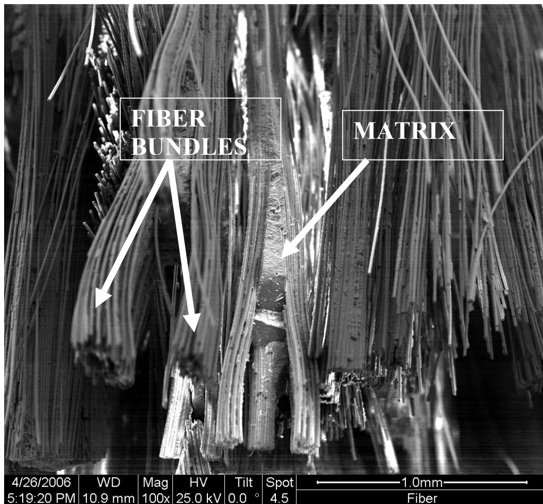
Figure 4. Micrograph of the N720/A specimen subjected to creep at 45 MPa in laboratory air. Fiber bundles and matrix are clearly seen.
