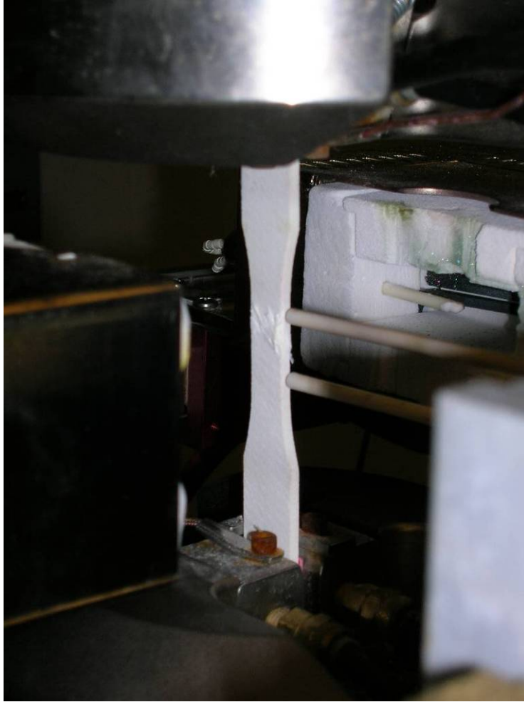
Figure 17. Extensometer on a fractured specimen.
