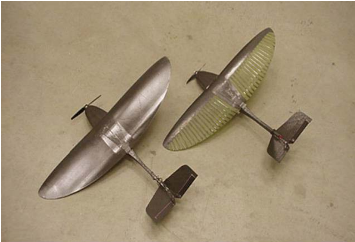
Figure 1. Rigid and Flexible Wing BATCAM V-Tail Variants (Photo courtesy of Dr. Richar Cobb, AFIT/ENY)
