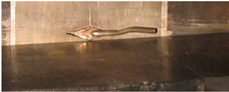
Figure 11. Moveable sidewall with diamond-shaped probe strut hole.
