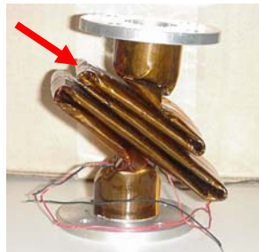
Figure 1.3-4: Folded Sub-T g Tube (Arrow Indicates Coldest Point – inside Fold)
