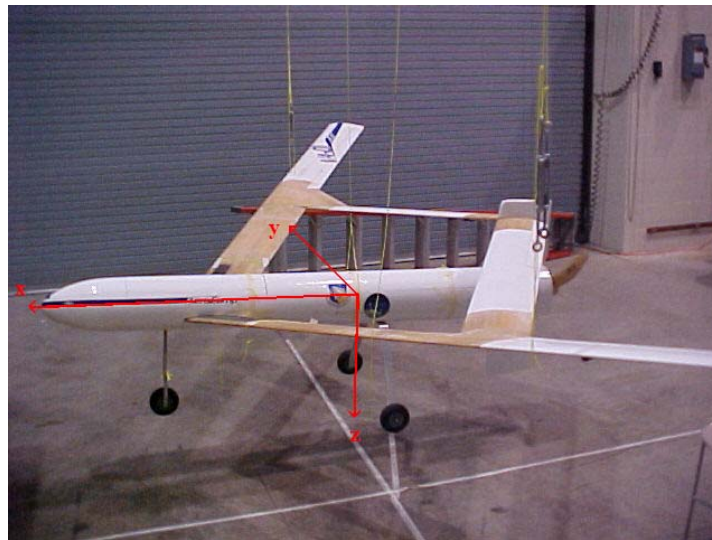
Figure 8. Center of Gravity Measurement with Body Axes Labeled.
