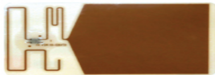
Figure 2: Passive RFID tag [Int04]
