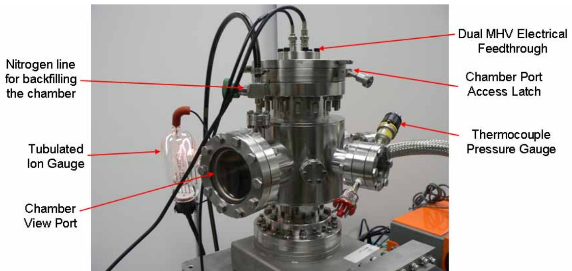
Depiction of the vacuum chamber showing the nitrogen line for backfilling the chamber, and the electrical feedthrough.
