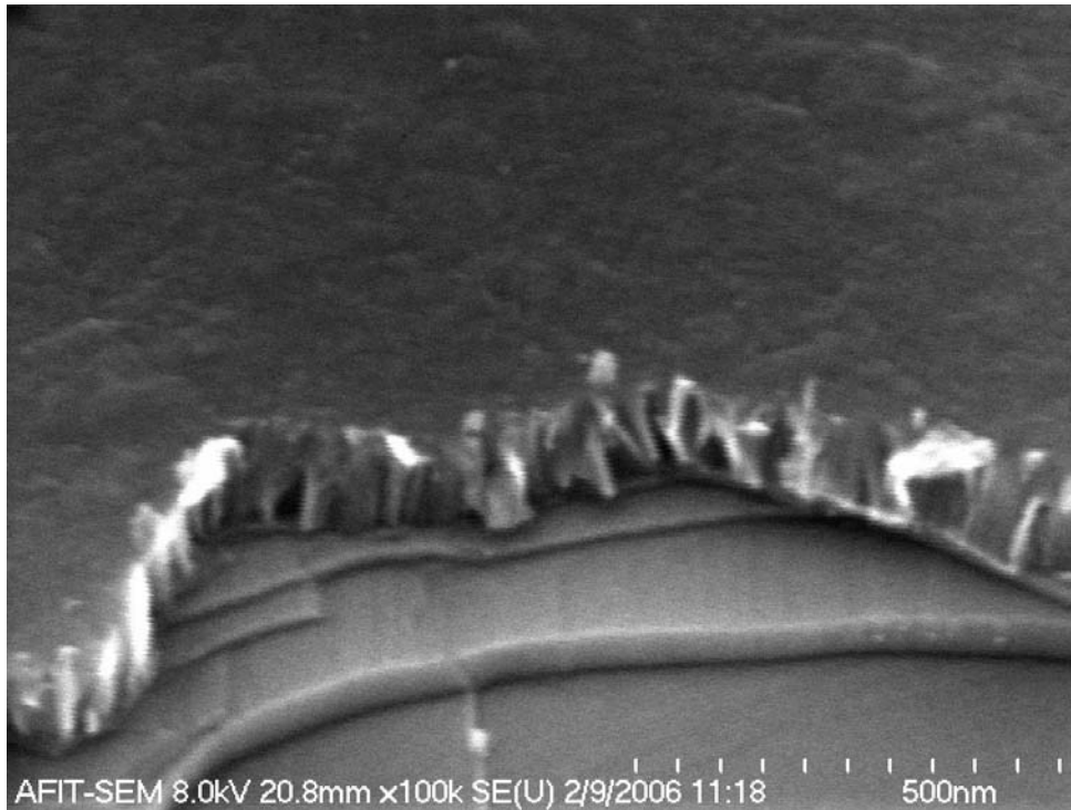
Figure 55. 100,000x magnification SEM image of a CNT film grown at 1700°C under 10^{-3} Torr vacuum pressure for 0.5-hours that did not undergo post-growth annealing (45° stage tilt).
