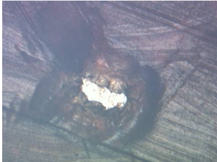
Figure 29. Non-circular hole in the Teflon ® film made using a 1/16" drill bit (5x magnification).
