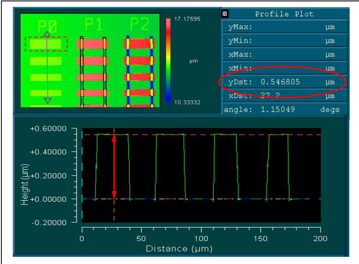
Figure 5-4. Optical profiler measurement to determine the thickness of the deposited polysilicon layer (Poly0). Note: the value shown is for only one measurement, and the reported values in Table 5-1 shows the average thickness values based on multiple measurements.
