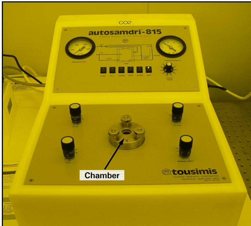
Figure A-2. Automatic supercritical CO 2 dryer used to prevent stiction in the MEMS dies used in this research effort.
