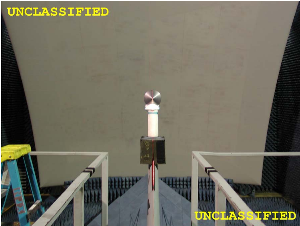
Figure 3-4: Large PEC cone on mount at AFRL compact RCS range
