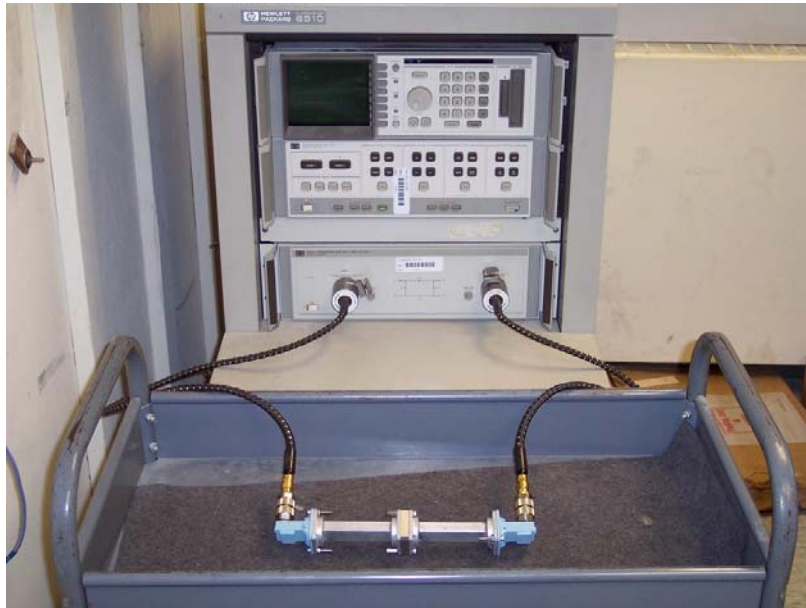
Figure 4-3. X-band waveguide WR90 attached to HP8510C Vector Network Analyzer with coaxial cables.
