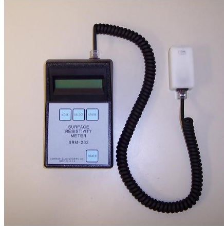
Figure 1-3. Guardian model SRM-232 four-point probe.
