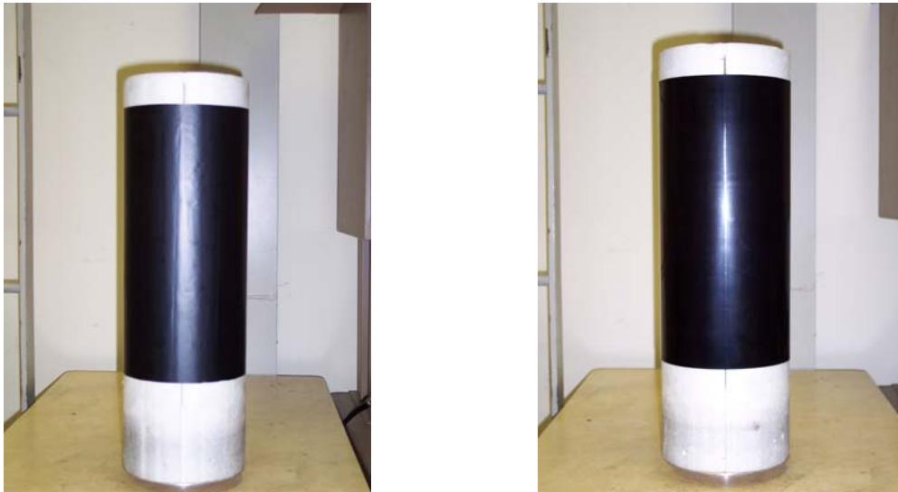
Figure 1-1. R-cards wrapped around a polystyrene foam cylinder. On the left is an R-card with a measured DC resistivity of 892 \Omega /sq. On the right is another R-card with a measured DC resistivity of 64 \Omega /sq.
