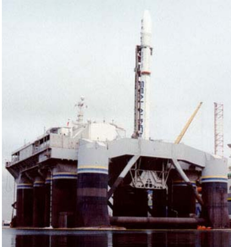
Figure 9: Zenit 3SL atop the Floating Launch Platform (Sea Launch Image Gallery)
