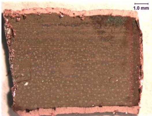
Figure G.53. Digital picture of the interior of copper recirculation pipe.
