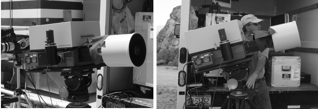
Figure 3.1: Two photos of the Bomem MR-254 Fourier Transform Spectrometer with the NFOV telescope at Edwards AFB, CA (see section 3.3). Also visible: the Cannon XL-2 video camera used to document tests (left) and AFIT technician Greg Smith (right).
