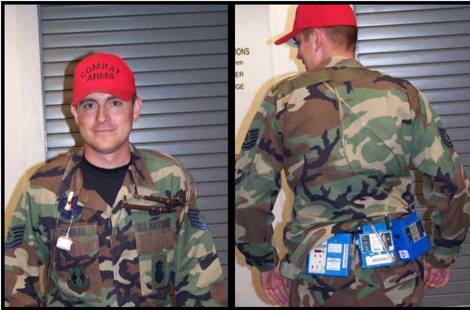
Figure 3.3 Personal Air Sampling Assembly to Capture Breathing Zone Contaminants
