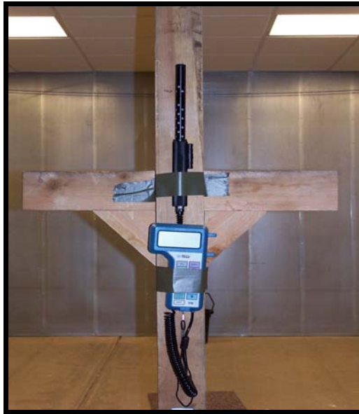
Figure 3.4 TSI Q-TRAK monitoring position. The CO monitor was positioned at station 8 on 21 Sep 05 and station 12 on 23 Sep 05 between two students to monitor CO levels during firing.
