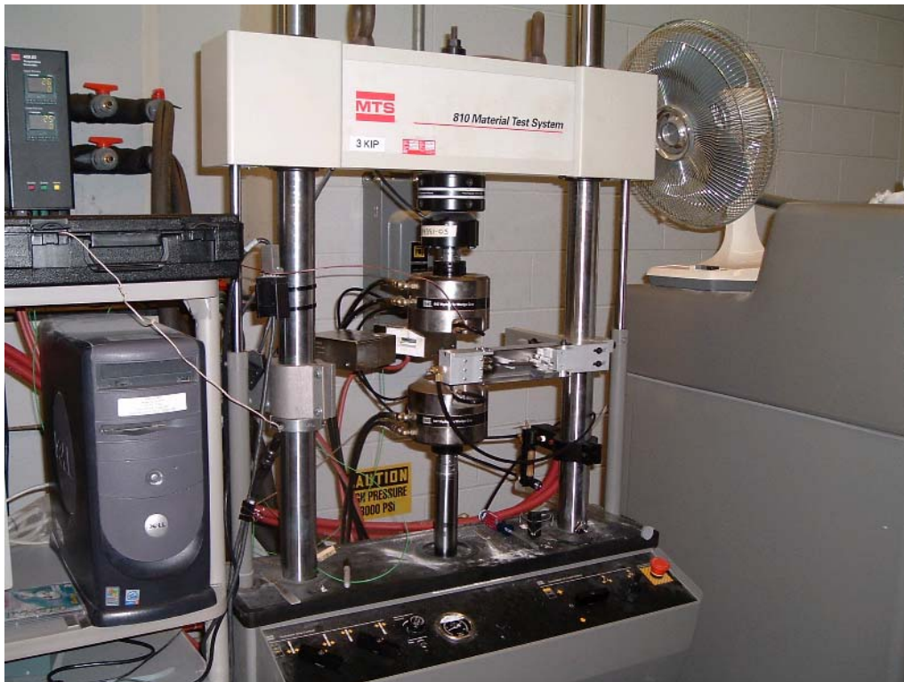
Figure 13: 3 KIP MTS Hydraulic Machine
