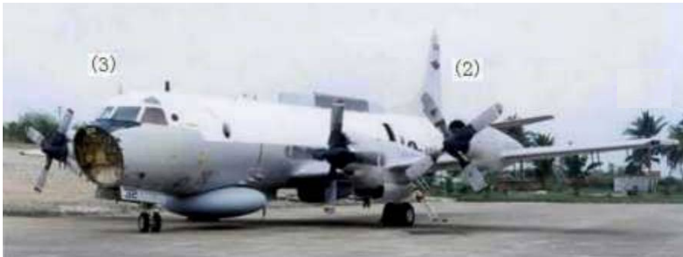
Figure 2. Captured EP-3E. Note the chipped propeller blade at (2) and the missing radome at (3). [Tri01]
