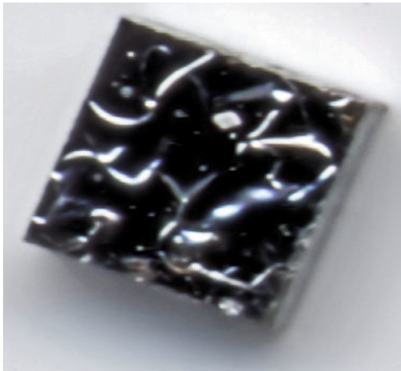
Figure 6-2 Test Chip with growth of GST at 9 \text{ \AA/s} to 4\text{-}\mu\text{m} thick (no usable devices).
