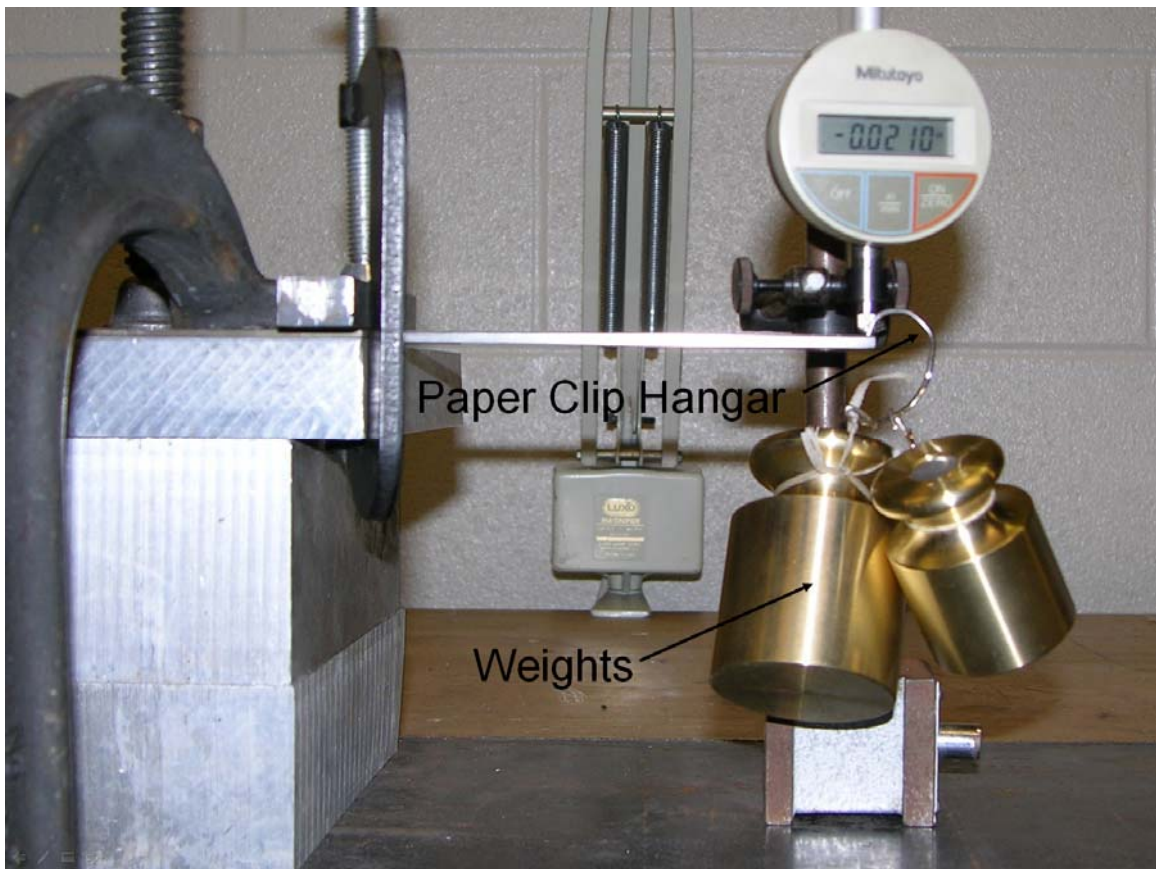
Figure 8. Cantilevered Beam with Weights Applied
