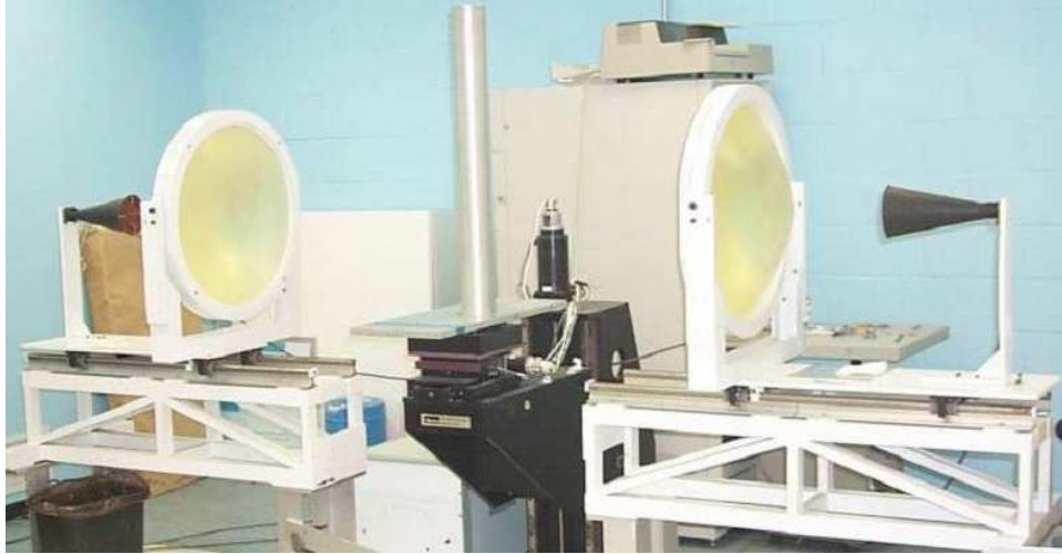
Figure 3.4: General Electric's focus arch free-space range with transmit horn on the left and receive horn on the right. The sample holder is not shown but is located in the middle, in place of the calibration cylinder shown.
