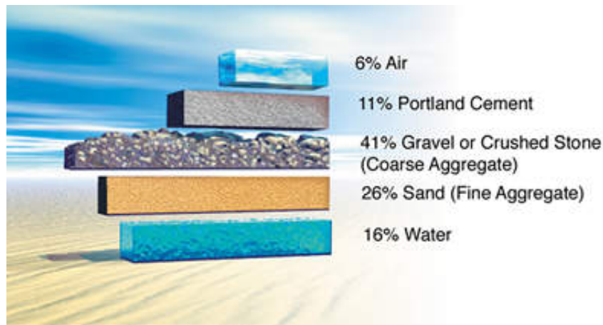
Figure 7: Concrete Components (PCA, 2005). Maintaining proper proportions of ingredients will help ensure high strength.
