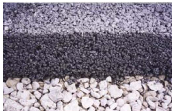
Figure 17: Cross-section of Porous Concrete (Offenburg, 2005). Porous concrete can be poured directly over a gravel base.
