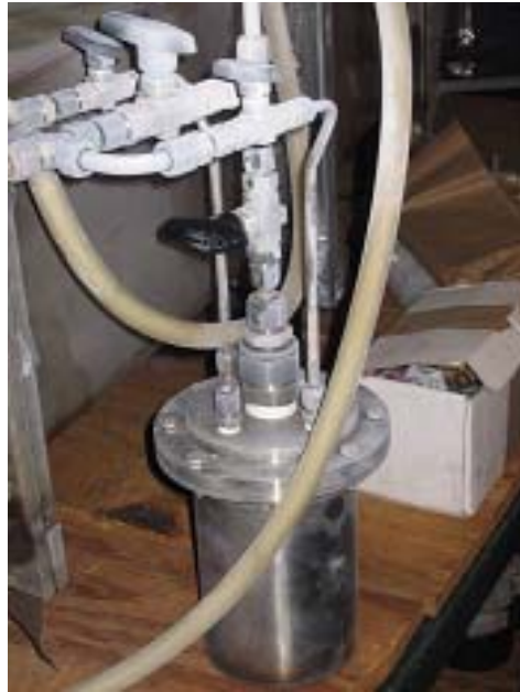
Figure 18. Photograph of cyclone seeder used for injecting aluminum oxide particles into air stream.
