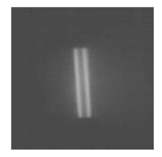
Figure 4.33: An image of the two filament like areas of the Newport/Oriel Hg(Ar) pencil lamp. The image was captured through the LCTF with a selected center wavelength of 546nm. The Ne source looks similar when imaged with the NIR filter.
