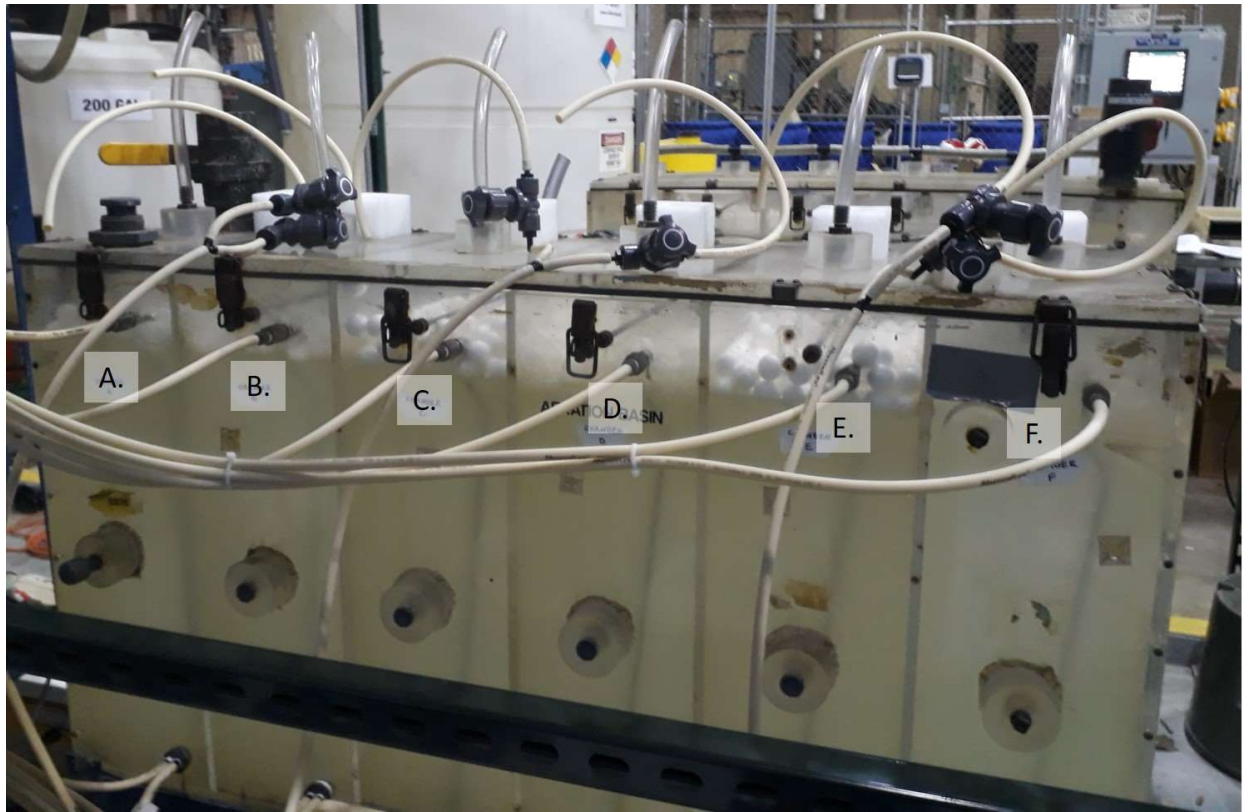
Figure 6. Aeration basin for the large-scale experimental setup composed of six separate compartments labelled A through F.
