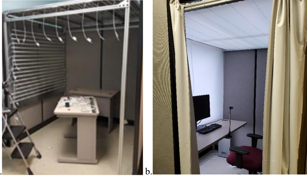
Figure 4. Photo of the Modified Cubicle Used in the Experiment (a) Without and (b) With the Diffusers and Curtain in Place
