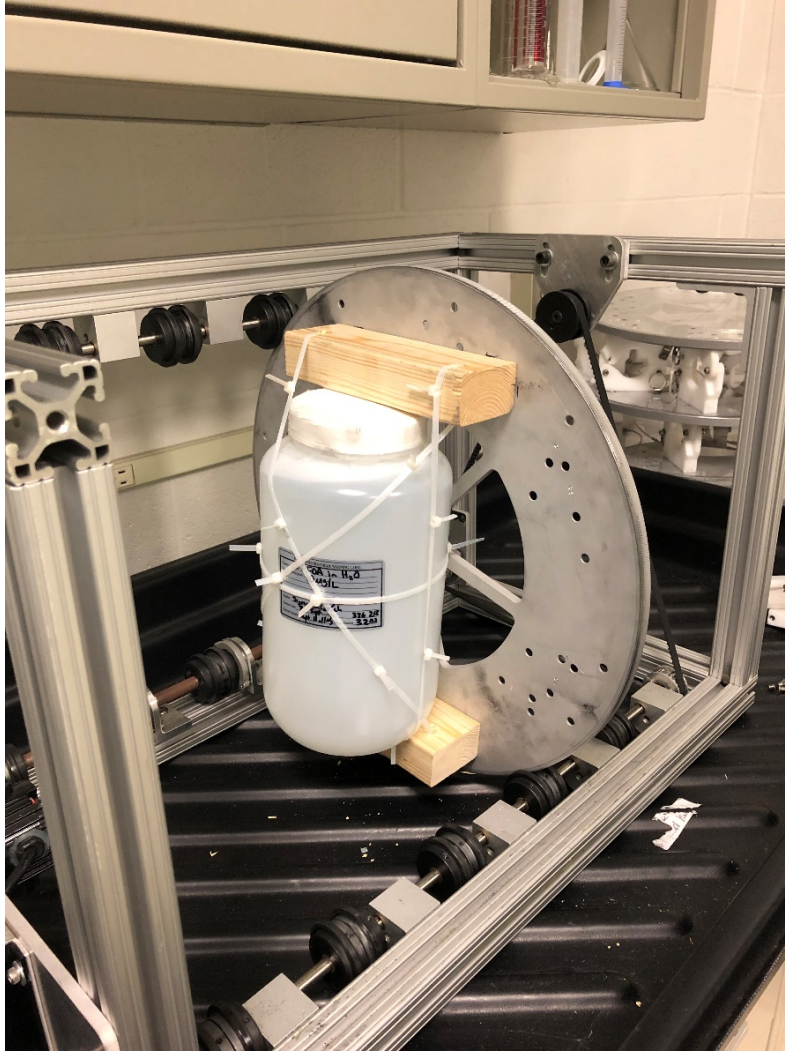
Figure 3-6: Automatic tumbler setup for the 4 L bottle with PFOA.
