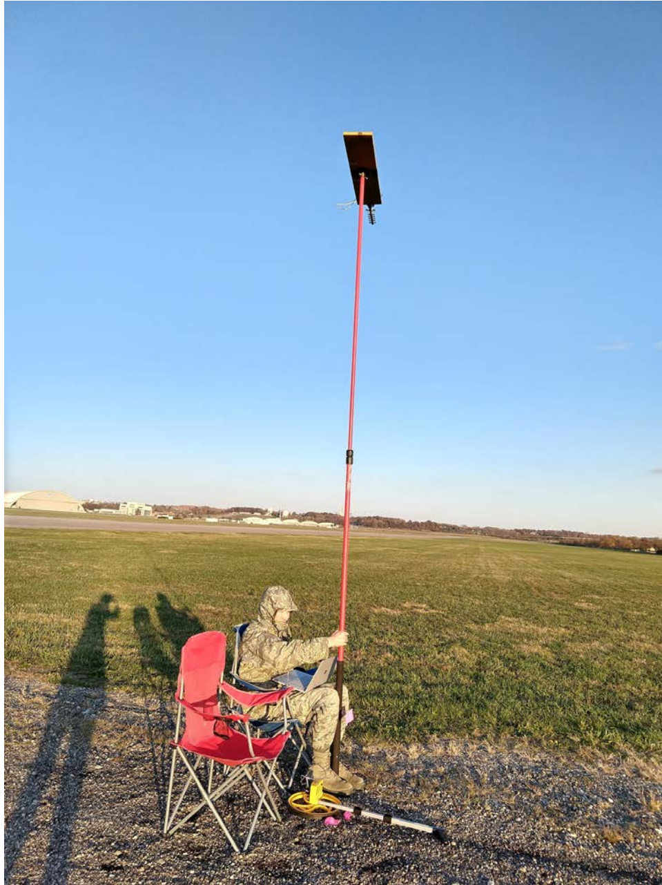
Figure 20: Conducting wireless attacks with skypie v2 at 1600 Meters
