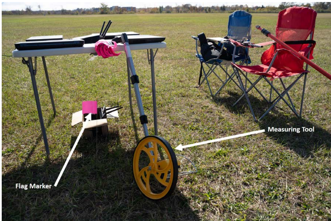
Figure 24: Flag markers and measuring tool
