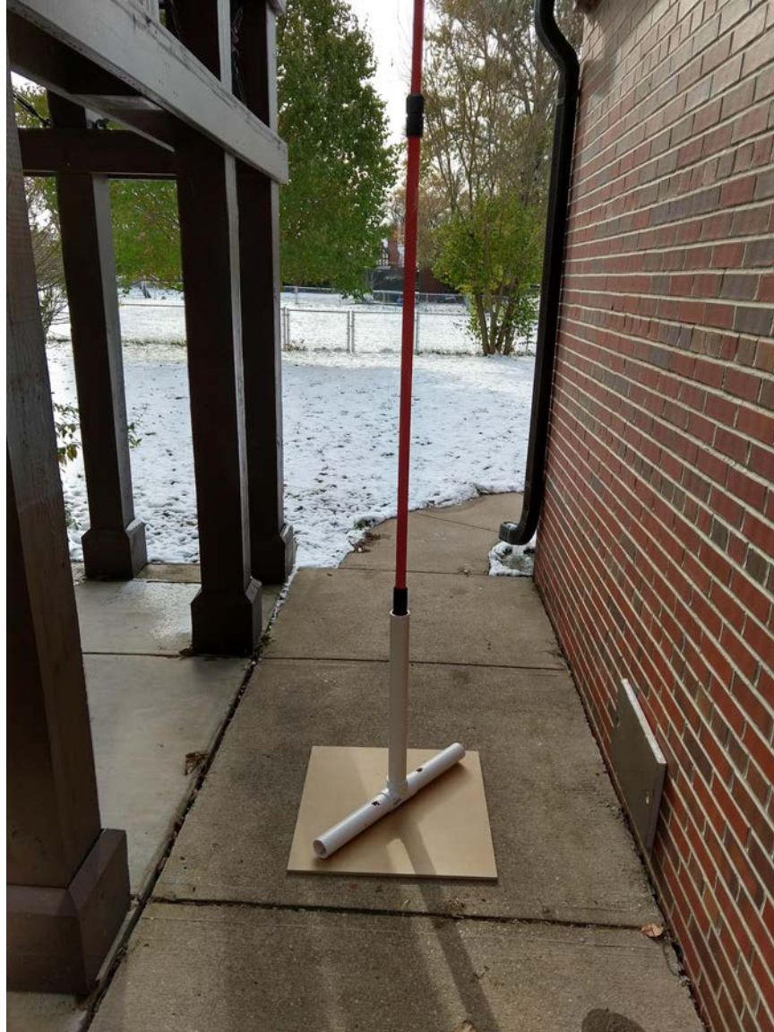
Figure 25: PVC sheath used to stabilize the mounted skyPie simulating drone flight
