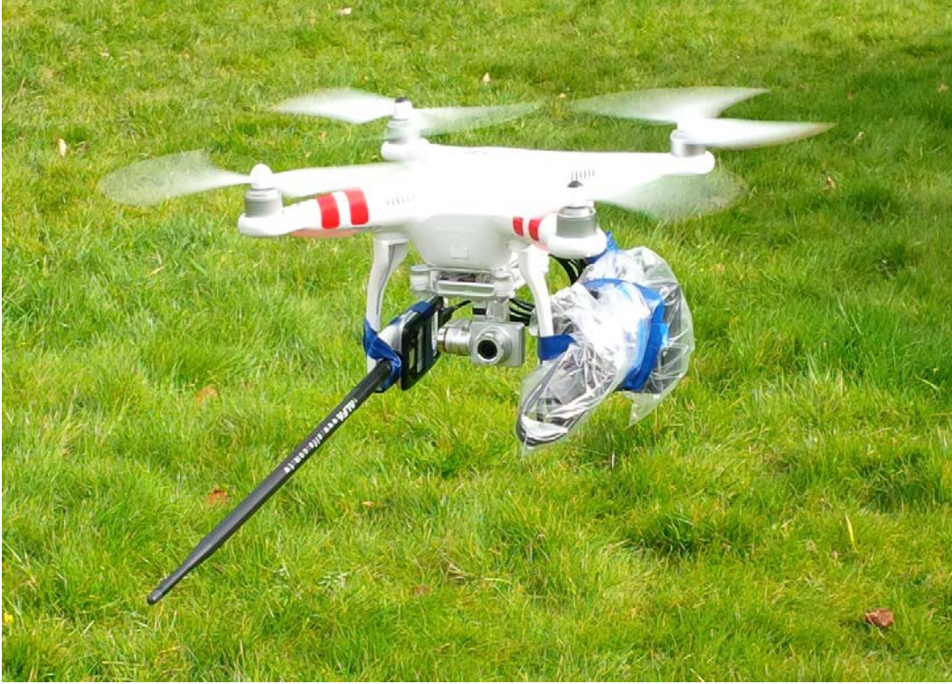
Figure 7: DJI Phantom 2 Vision+ with wireless attack payload [51]
