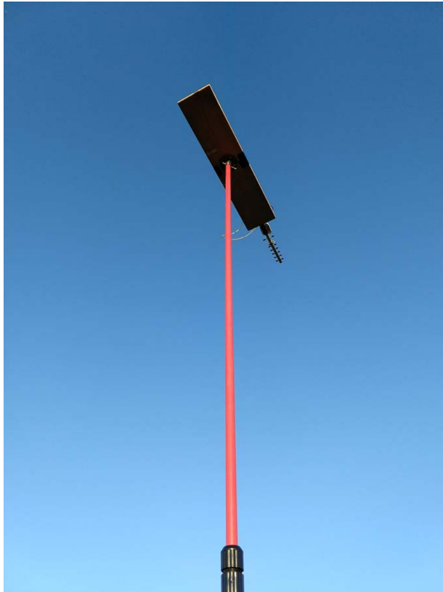
Figure 22: “Simulated drone flight”: skypie v2 platform mounted on telescoping pole via iron pipe fittings
