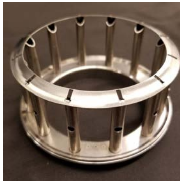
(b) The back plate with fuel-air mixing tubes and impingement plate welded.
