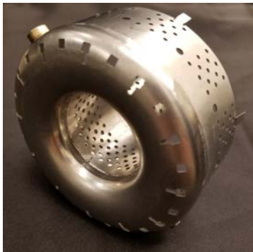
(a) The forward dome with inner and outer diameters welded.
