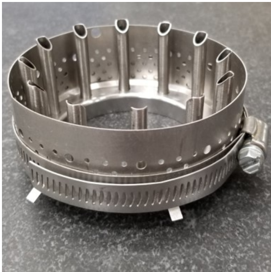
(a) Outer diameter pictured with the back plate and fuel-air mixing tubes.
