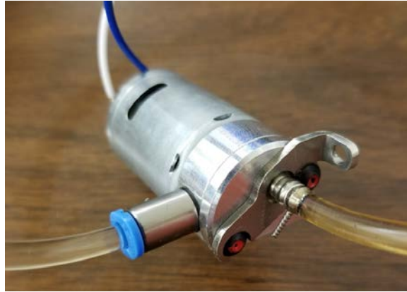
Figure 43. The pump used to flow lubrication to the JetCat P90 RXi during rotating testing.
