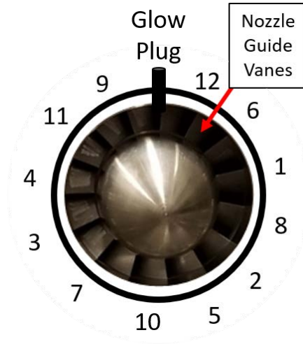
Figure 44. The rearranged propane line placement around the engine as viewed from the rear of the engine with glow plug and turbine nozzle guide vanes for reference.
