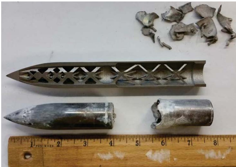
Figure 8. Graves' projectile failed similarly to Richards'.
