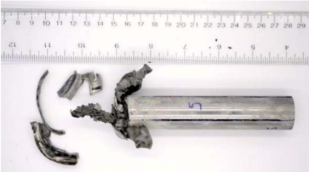
Figure 13. Patel's Projectile catastrophically failed by having the nose splintering on impact with the targets. The insert can be seen surviving at the midpoint of the projectile.
