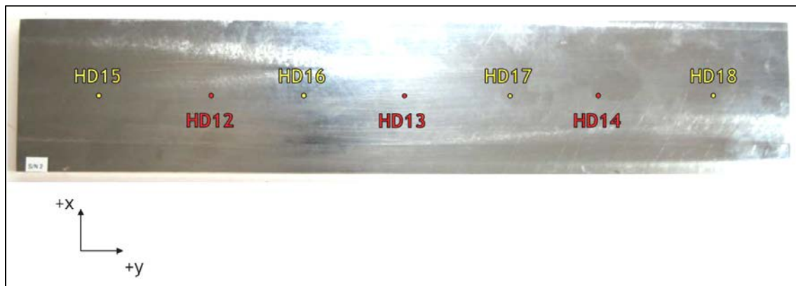
Figure 26: Representative titanium plate and hole-drilling locations (LSP treated spots in yellow and far field baseline locations in red) [105]
