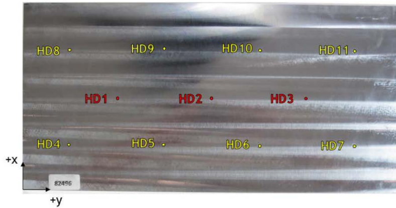
Figure 2: Representative diagram of hole drilling measurement locations for specimens: 82495 and 82496.
