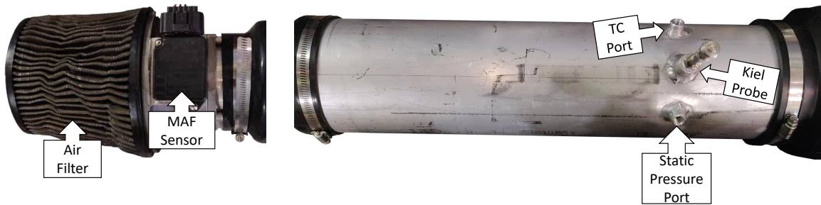
Figure 56. Test Stand Compressor Filter, MAF, and Intake.
