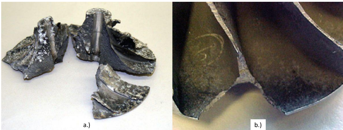
Figure 11. Centrifugal Compressor Failure. a.) Bore Failure. b.) Outer Blade Tip Failure [25]
