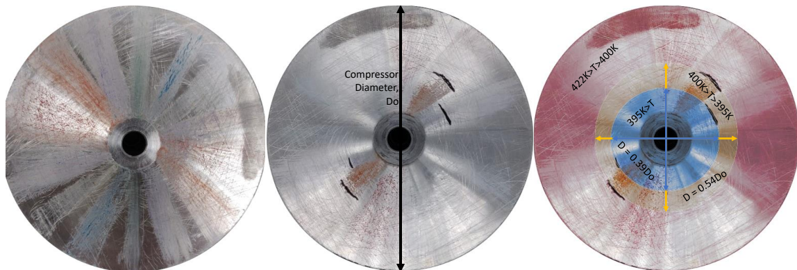
Figure 98. GTX5008R Back Face Heat Map. Before Test (left). After Test (middle). Digitally Colored (right).
