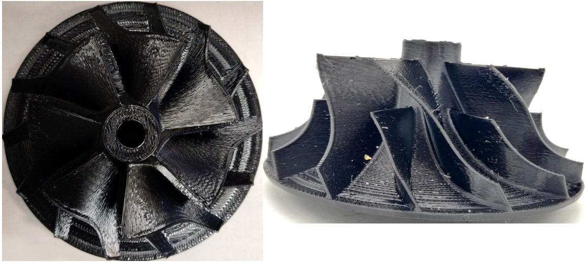
Figure 100. Printed Modified P400 Compressor, ULTEM 9085
