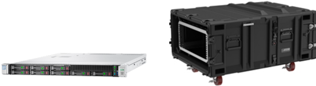
Figure 9: Typical high performance network sensor server with an “airline approved” hard sided transit case. Typical airline restrictions limit special checked items like this to 100 lbs [65]
