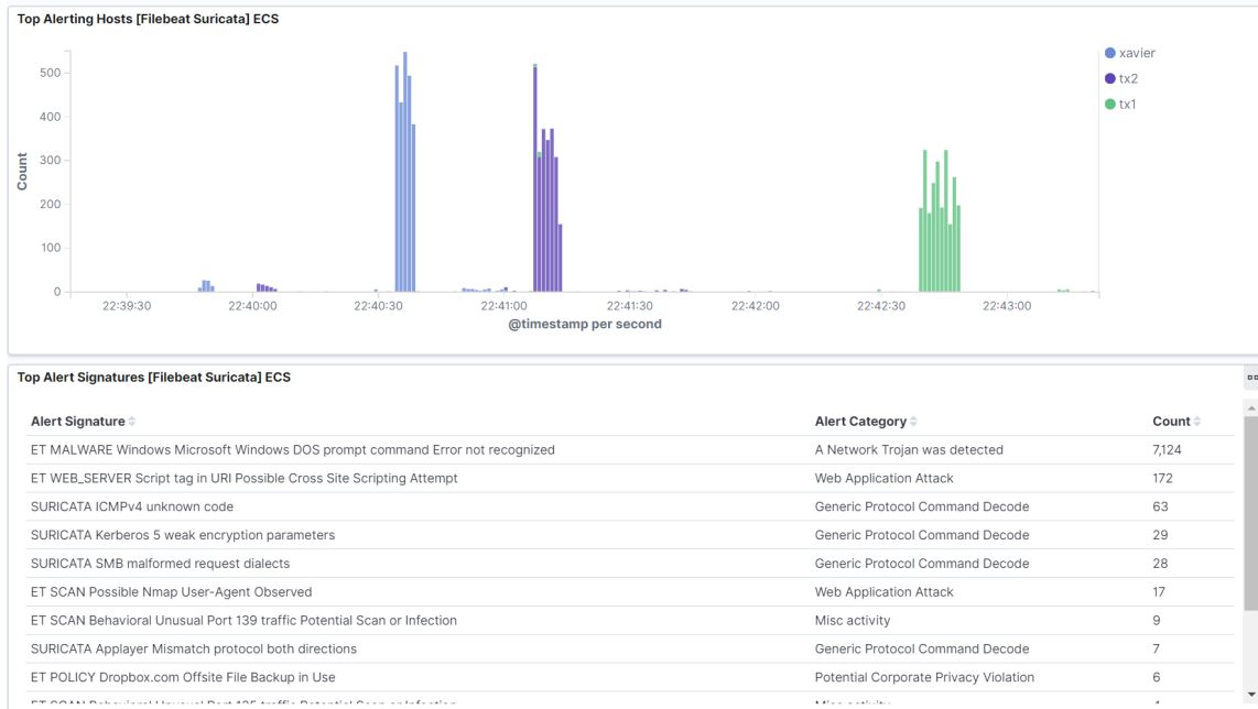
Figure 52: Kibana Dashboard with all alerts reporting. The timestamps are different due to slight wall clock drift between devices
