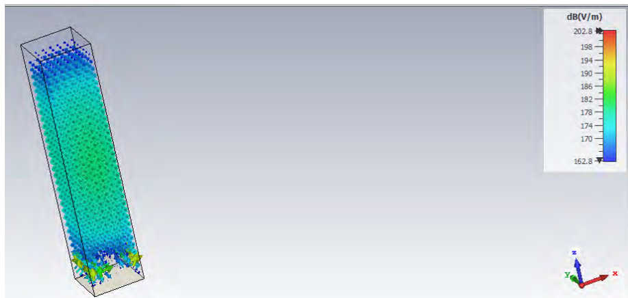
Figure 52: Fractal Unit Cell: Mode 4 E Field, g = 0.2 mm, \phi = 80^\circ
