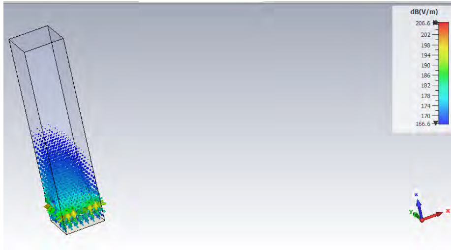
Figure 51: Fractal Unit Cell: Mode 1 E Field, g = 0.2 mm, \phi = 80^\circ
