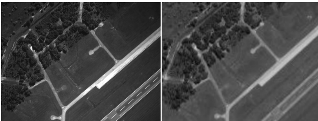
Figure 3: Left shows the real world imagery taken from the SUSEX Flight 12 dataset. Right shows the equivalent imagery created in the AftrBurner Engine.
