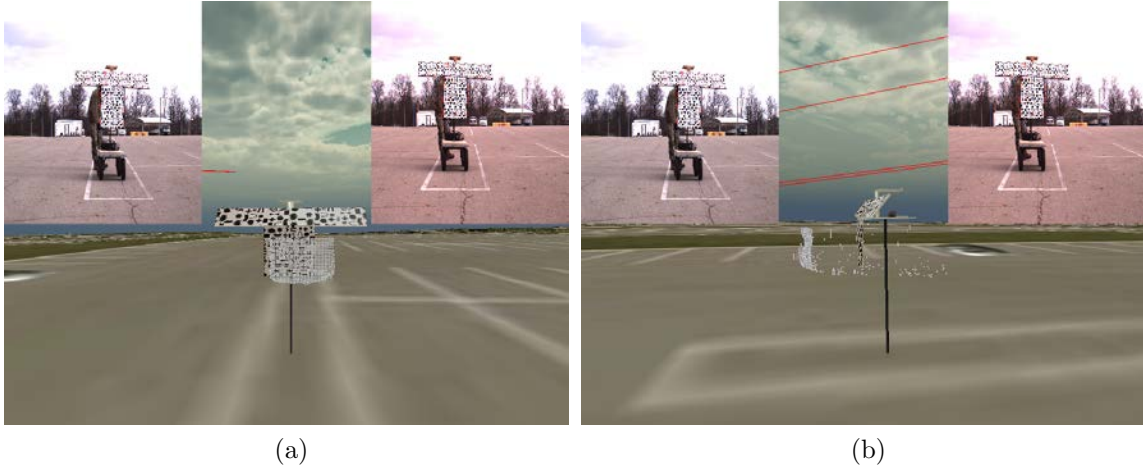
Figure 14. The real 3D point cloud after medianBlur
