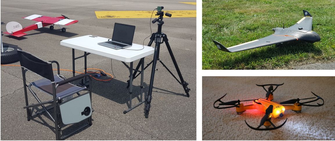
Figure 52: (Left) Equipment setup to track drones at Wright-Patterson Air Force Base with the fixed wing drone in the background. (Top right) The Skywalker x8. (Bottom right) The SS40 quadcopter with front and rear LEDs.
