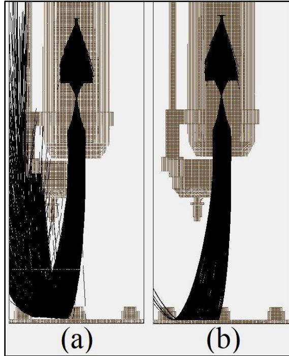
Figure 112: Electron trajectories (shown in black) for a spacing of 45.37 mm. The accelerating potentials were 195 V (a) and 204 V (b). All other potentials were set in accordance with Table 8.
