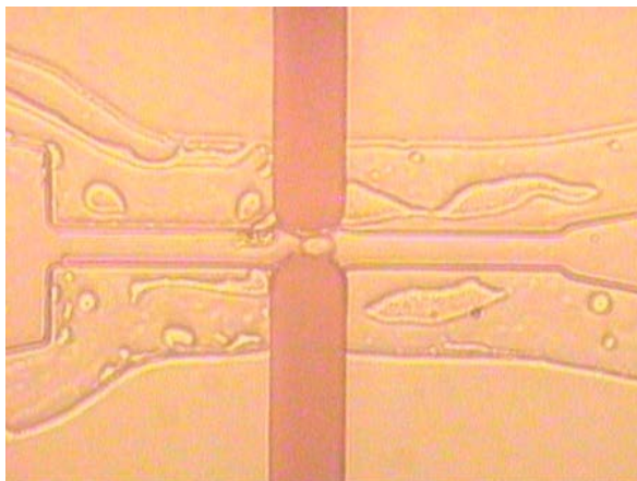
Figure 4.22 This micrograph zooms in on the microchannel of MC-05 during a cell impedance experiment. A single Jurkat T cell is shown between the microelectrodes.
