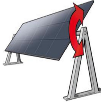
Figure 1. Single Axis Solar Tracking
