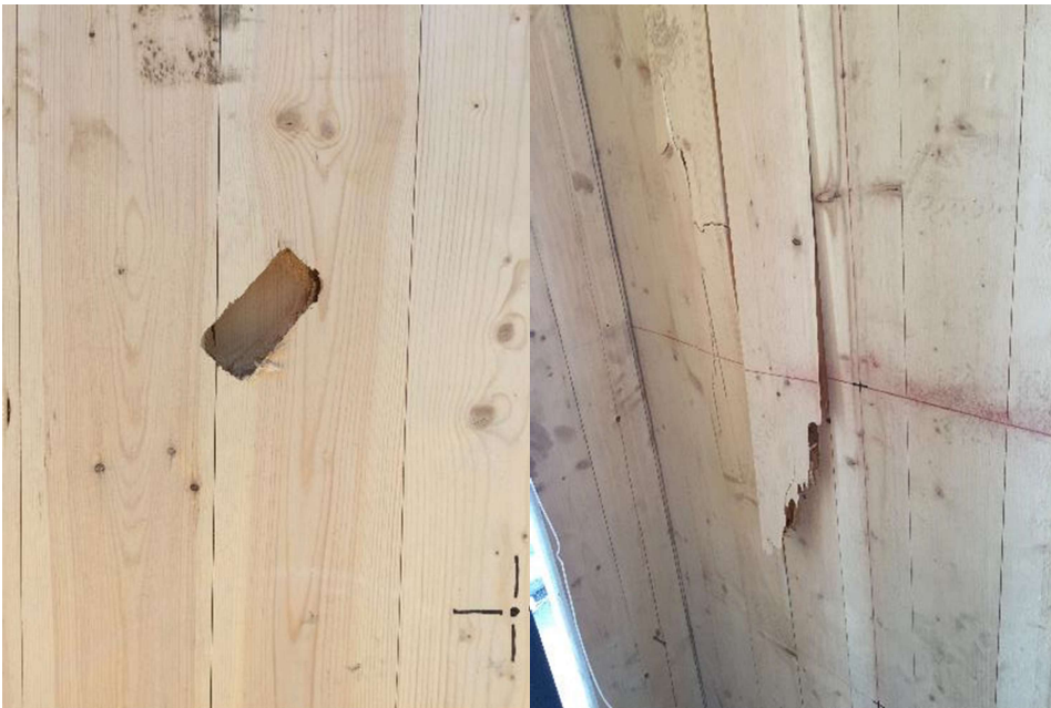
Figure A-11: Panel 4, weak-axis, strong-connection, edge, 12-pound, 100.2 mph, passed (front-left, back-right)
