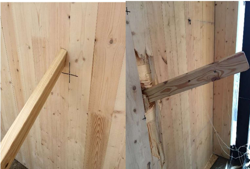
Figure A-7: Panel 3, weak-axis, strong-connection, center, 15-pound, 87.6 mph, failed – perforation (front-left, back-right)
