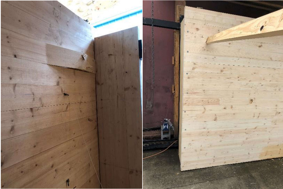
Figure A-24: Panel 8, strong-axis, strong-connection, corner, 15-pound, 110.2 mph, passed (back-left, front-right)
