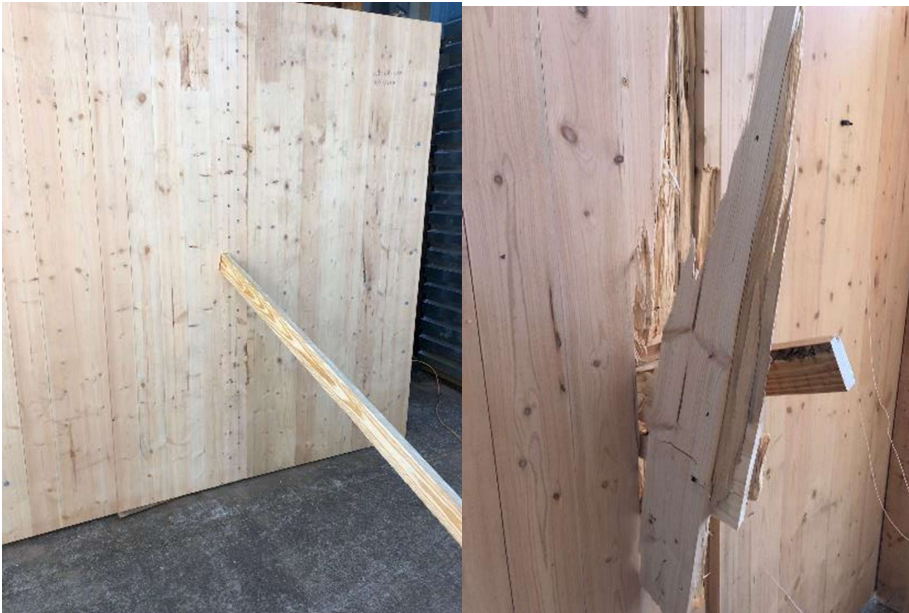
Figure A-43: Panel 15, weak-axis, half-lap connection, center, 15-pound, 87.7 mph, failed – perforation/dislodgement (front-left, back-right)
