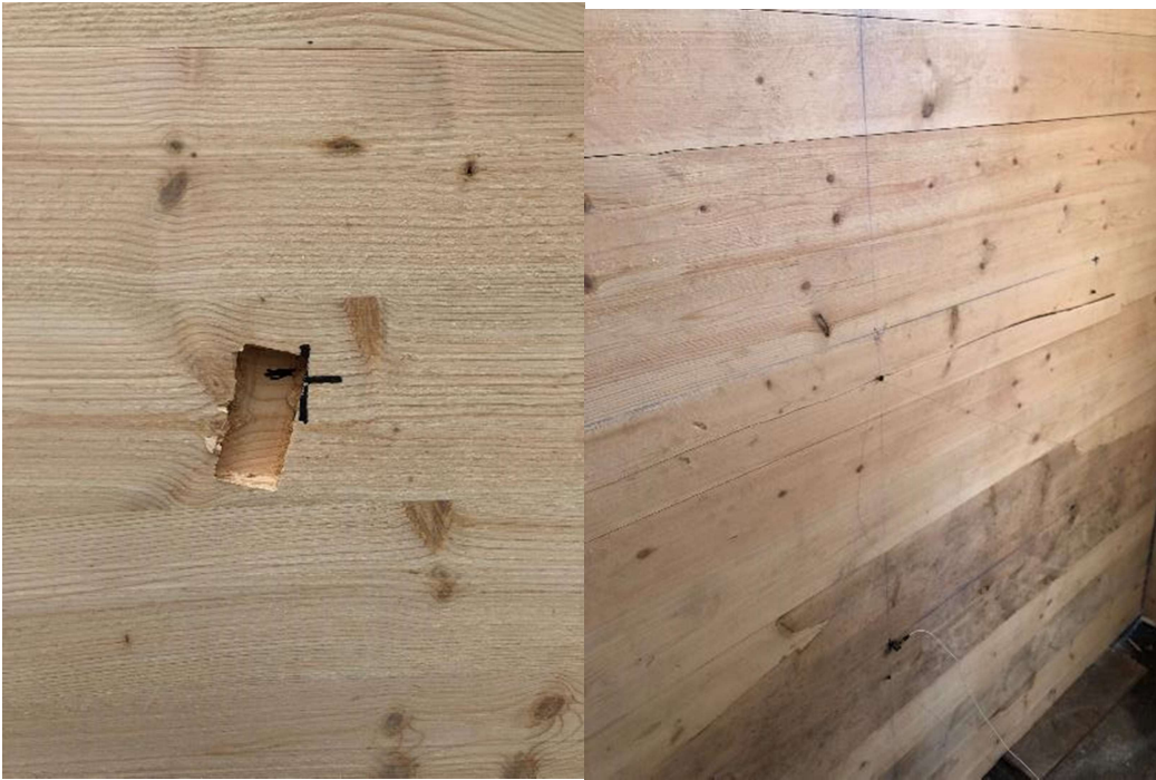
Figure A-22: Panel 8, strong-axis, strong-connection, center, 15-pound, 102.1 mph, passed (front-left, back-right)
