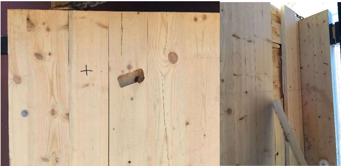
Figure A-21: Panel 7, weak-axis, strong-connection, corner, 15-pound, 89.9 mph, failed – dislodgement (front-left, back-right)
