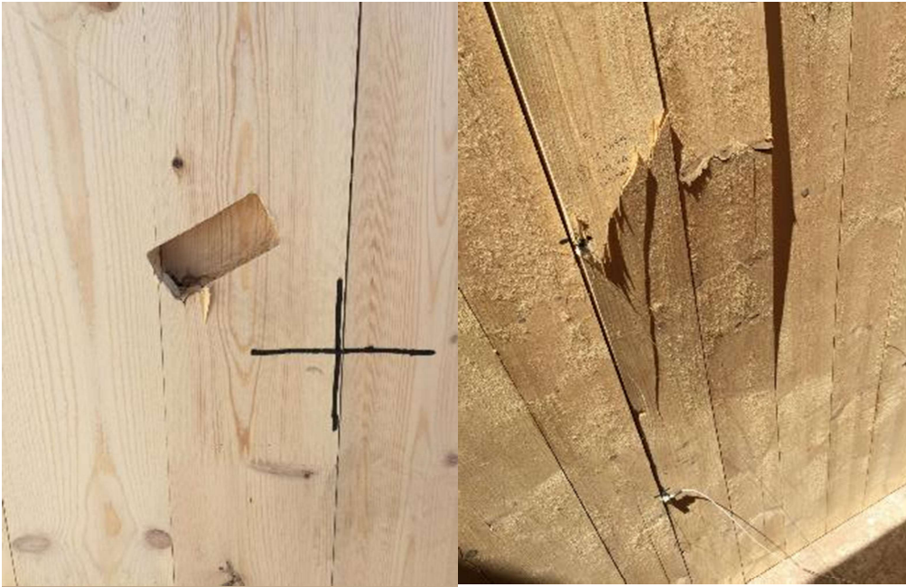
Figure A-4: Panel 2, weak-axis, strong-connection, center, 15-pound, 89.4 mph, passed test (front-left, back right)
