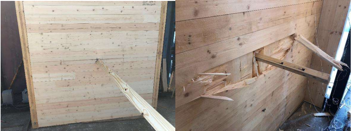
Figure A-28: Panel 10, strong-axis, weak-connection, center, 15-pound, 104.3 mph, failed – perforation/dislodgement (front-left, back-right)
