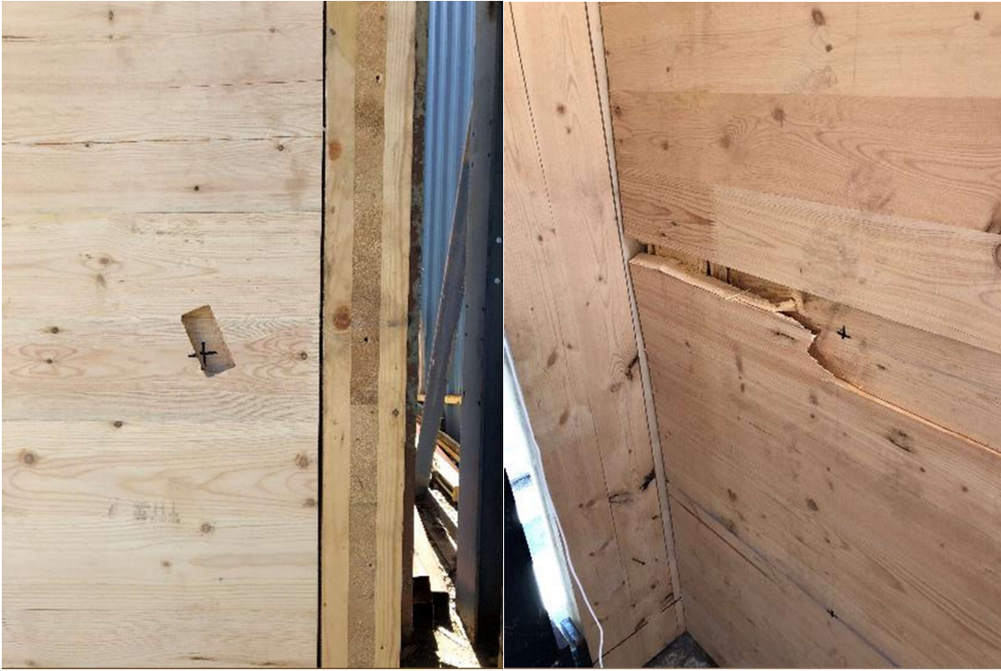
Figure A-26: Panel 9, strong-axis, weak-connection, edge, 15-pound, 93.9 mph, passed (front-left, back-right)
