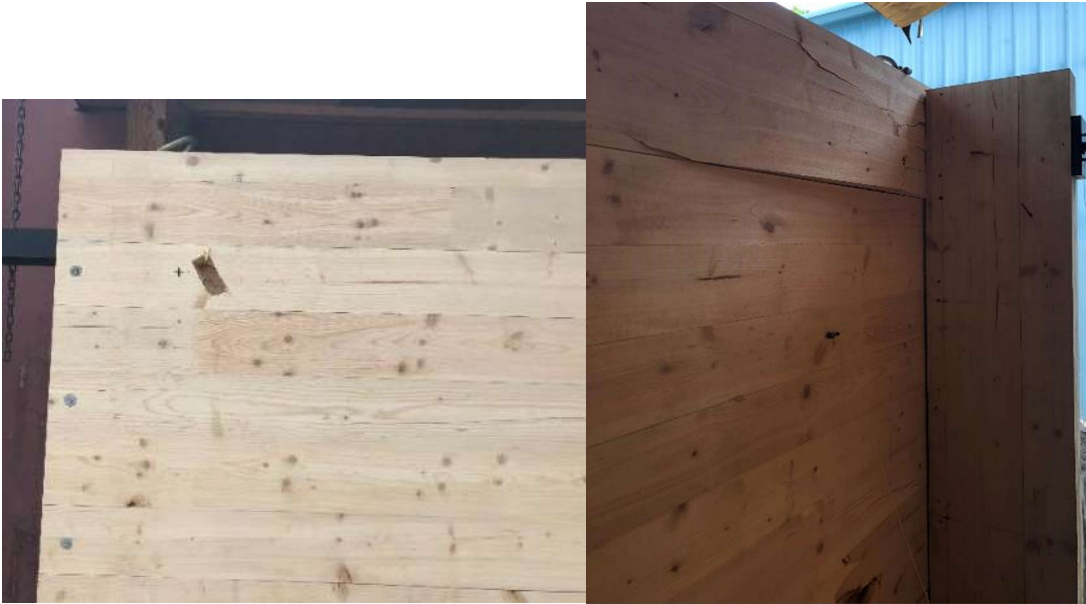
Figure A-36: Panel 12, strong-axis, strong-connection, corner, 14.5-pound, 103.9 mph, passed (front-left, back-right)
