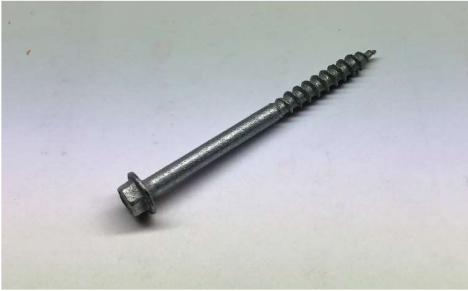
Figure 4.1: Simpson SD10212 screw tested in shear
