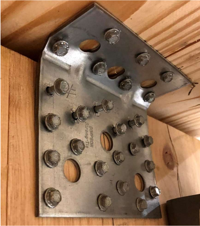
Figure 4.35: Deformation of AE116 at the top of out-of-plane wall
