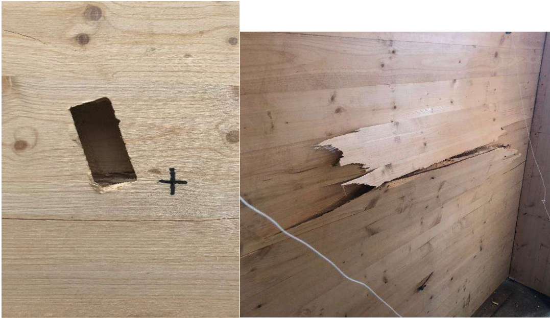
Figure A-34: Panel 12, strong-axis, strong-connection, center, 14.5-pound, 96.9 mph, passed (front-left, back-right)
