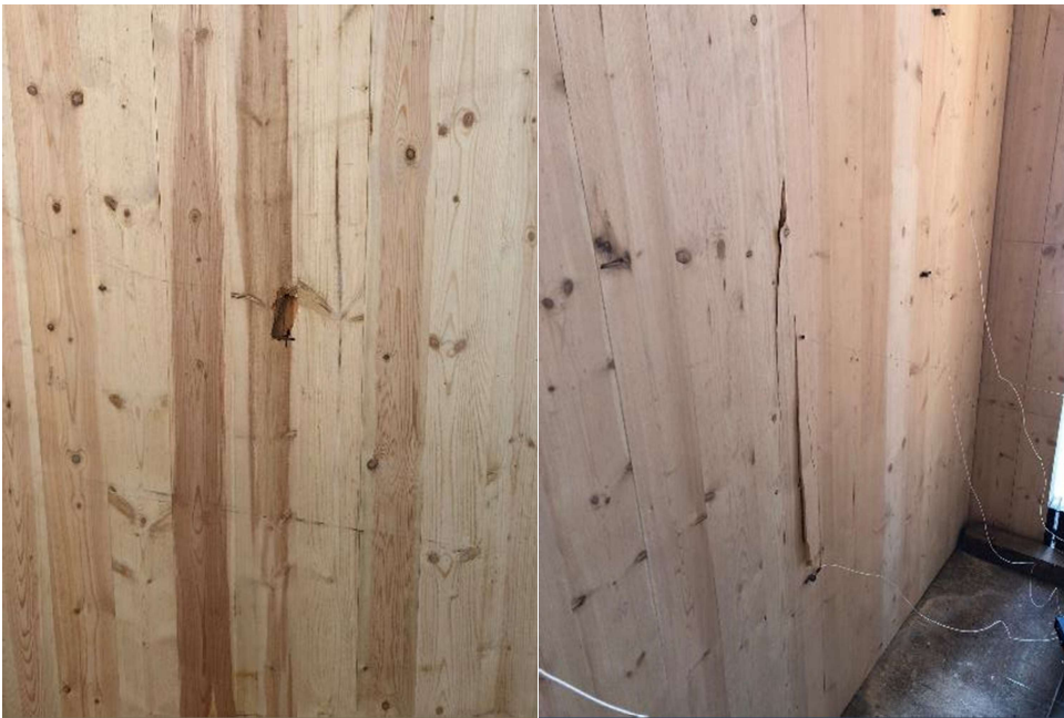
Figure A-37: Panel 13, weak-axis, weak-connection, center, 15-pound, 87.8 mph, passed (front-left, back-right)
