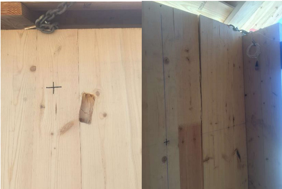
Figure A-15: Panel 5, weak-axis, strong-connection, corner, 15-pound, 88.0 mph, passed (front-left, back-right)
