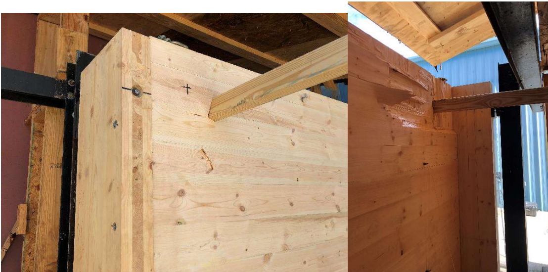
Figure A-27: Panel 9, strong-axis, weak-connection, corner, 15-pound, 101.6 mph, failed – perforation/dislodgement (front-left, back-right)
