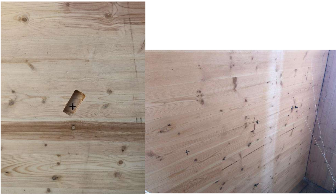
Figure A-31: Panel 11, strong-axis, strong-connection, center, 9-pound, 96.9 mph, passed (front-left, back-right)
