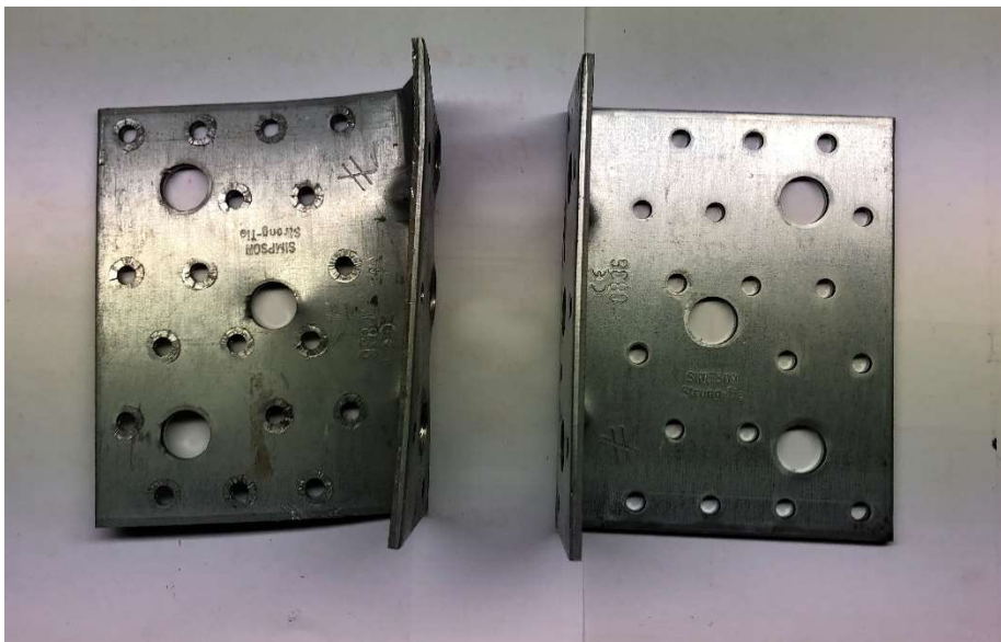
Figure 4.10: Comparison of deformed shape after cyclic loading (left) with undeformed shear bracket (right)
