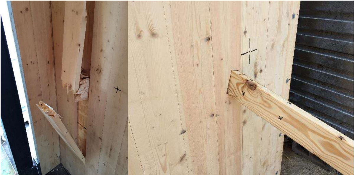
Figure A-8: Panel 3, weak-axis, strong-connection, edge, 15-pound, 88.1 mph, failed – permanent deflection (back-left, front-right)
