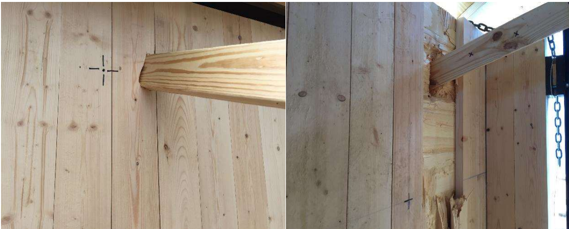
Figure A-9: Panel 3, weak-axis, strong-connection, corner, 15-pound, 91.9 mph, failed - perforation (front-left, back-right)
