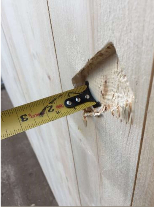
Figure A-2: Panel 1, weak-axis, strong-connection, edge, 15-pound, 59.4 mph, passed test (front of panel)
