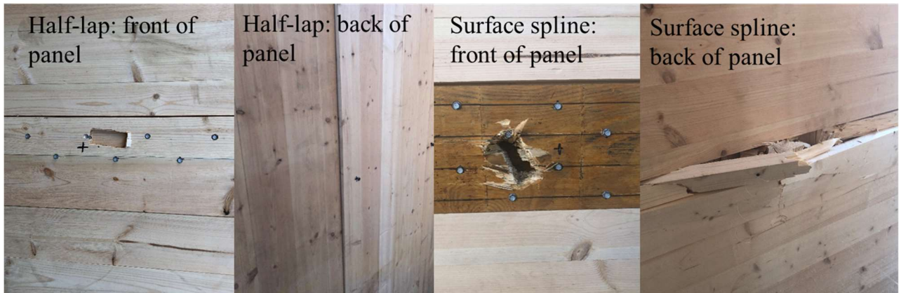
Figure 3.14: Damage photos of panel-to-panel connection tests
