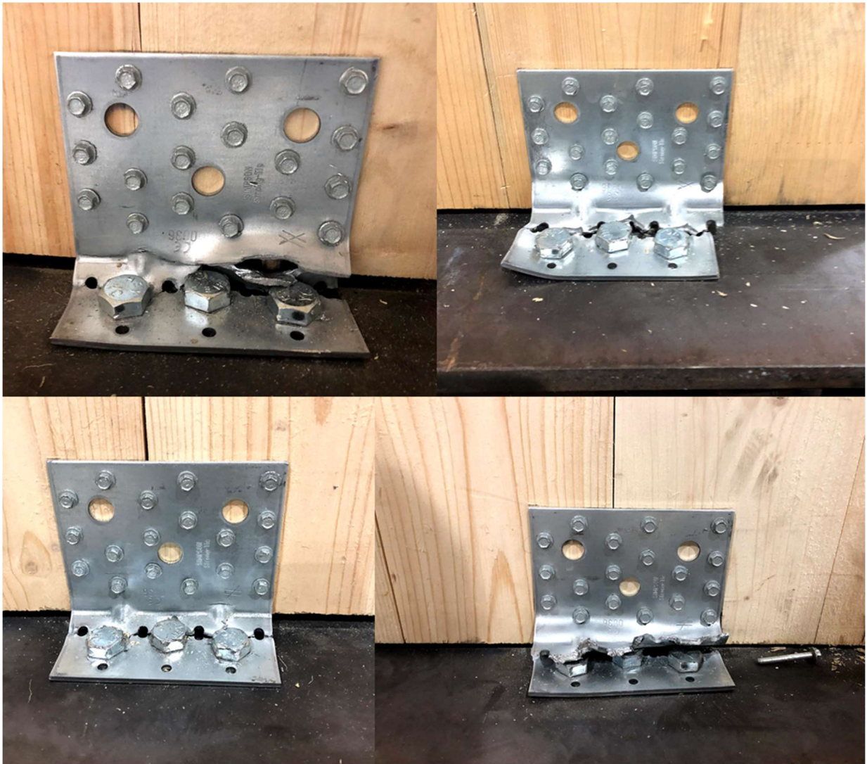
Figure 4.32: Failure of AE116 connections at the bottom of in-plane walls
