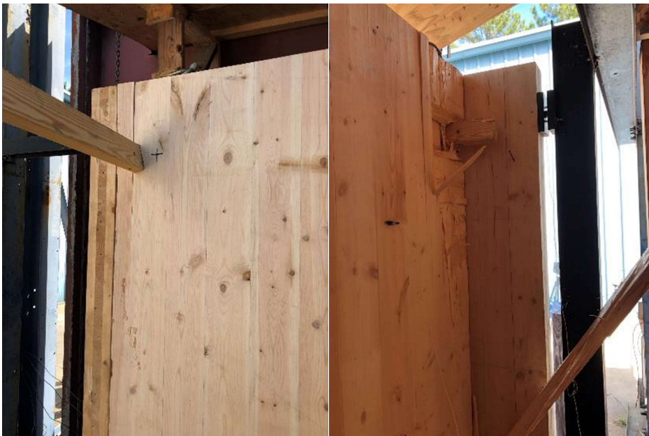
Figure A-39: Panel 13, weak-axis, weak-connection, corner, 15-pound, 89.4 mph, failed – perforation/dislodgement (front-left, back-right)
