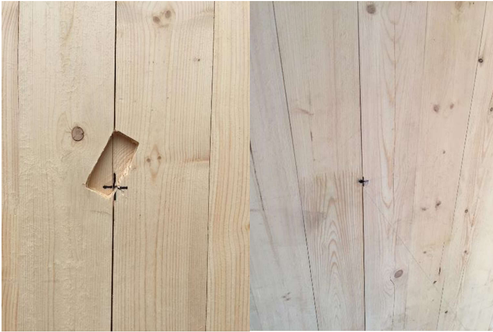
Figure A-16: Panel 6, weak-axis, strong-connection, center, 12-pound, 75.2 mph, passed (front-left, back-right)
