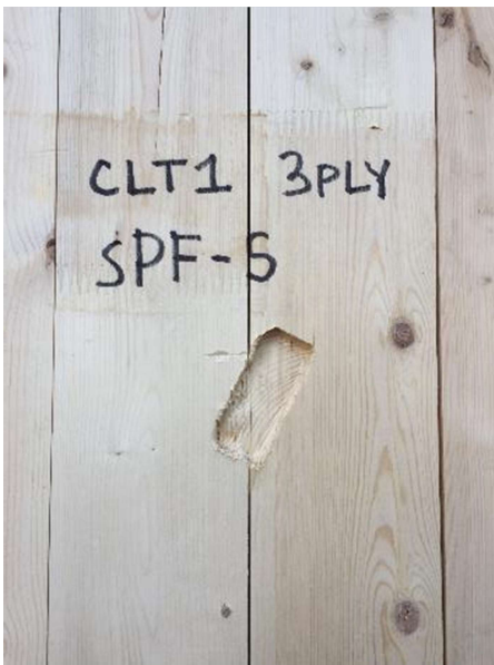
Figure A-3: Panel 1, weak-axis, strong-connection, corner, 15-pound, 62.2 mph, passed test (front of panel)
