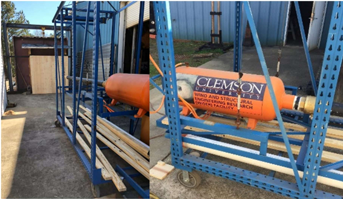
Figure 3.1: Pneumatic cannon used for experimental debris impact testing
