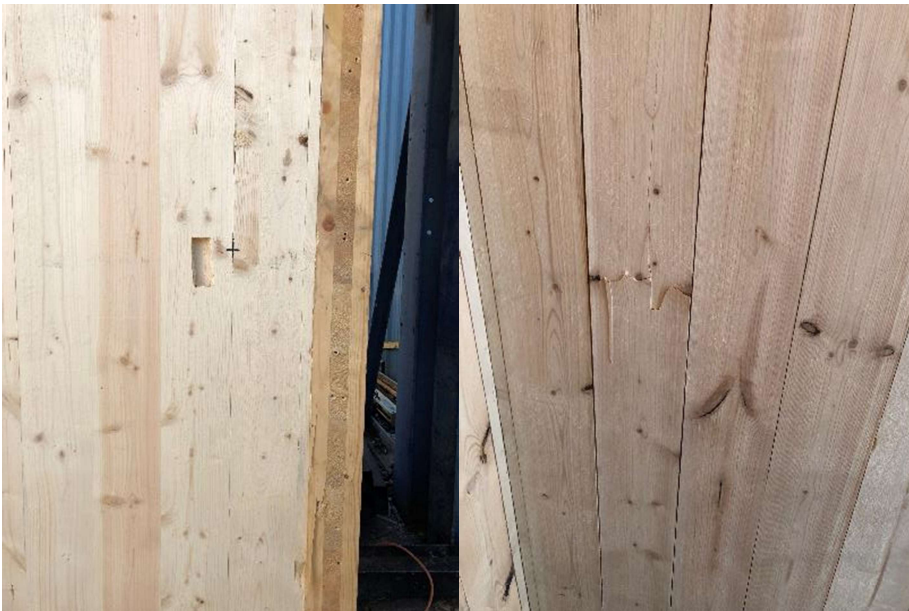
Figure A-41: Panel 14, weak-axis, weak-connection, edge, 9-pound, 79.5 mph, passed (front-left, back-right)
