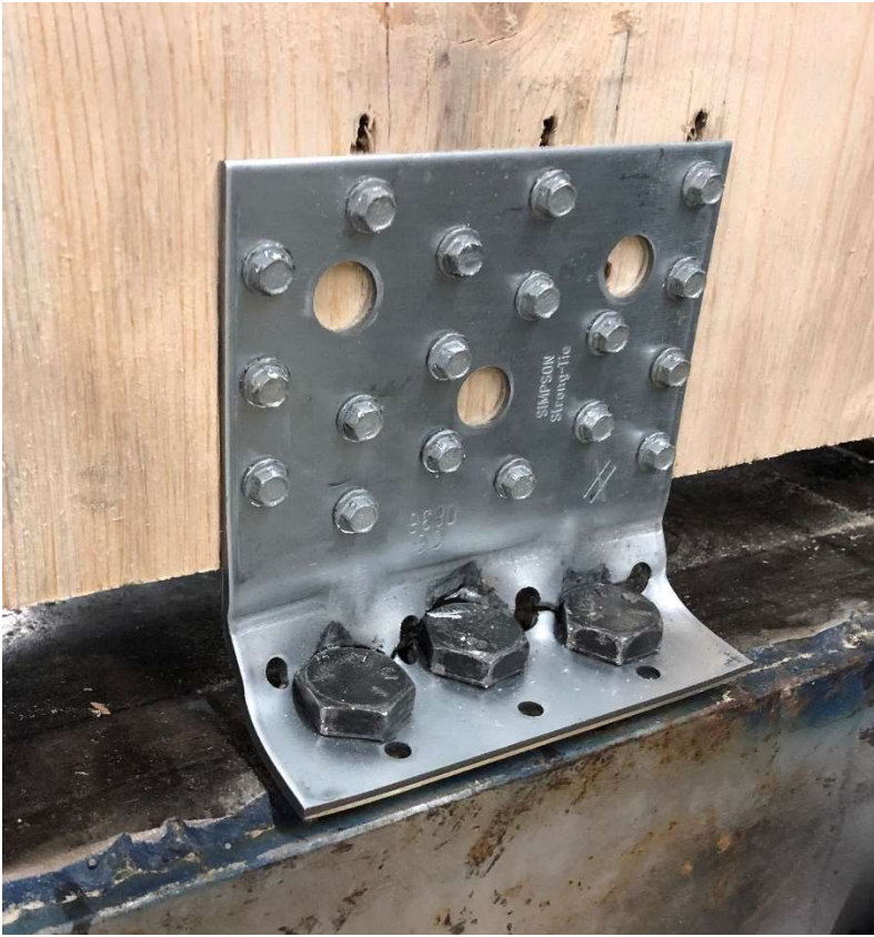
Figure 4.6: Monotonic uplift testing failure
