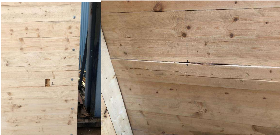
Figure A-23: Panel 8, strong-axis, strong-connection, edge, 15-pound, 119.4 mph, passed (front-left, back-right)
