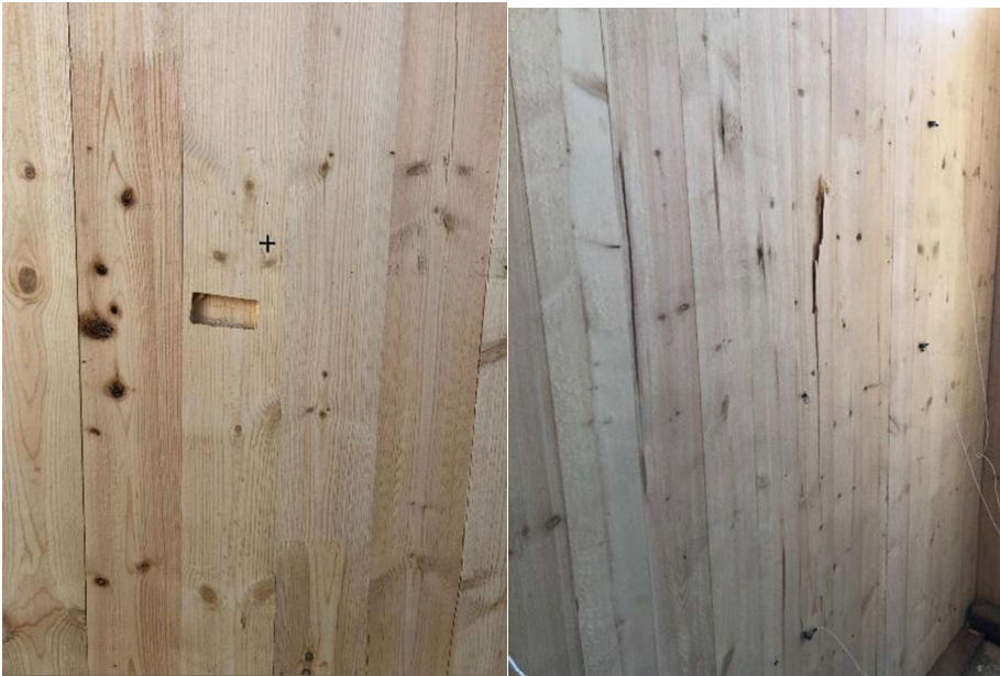
Figure A-40: Panel 14, weak-axis, weak-connection, center, 9-pound, 88.8 mph, passed (front-left, back-right)
