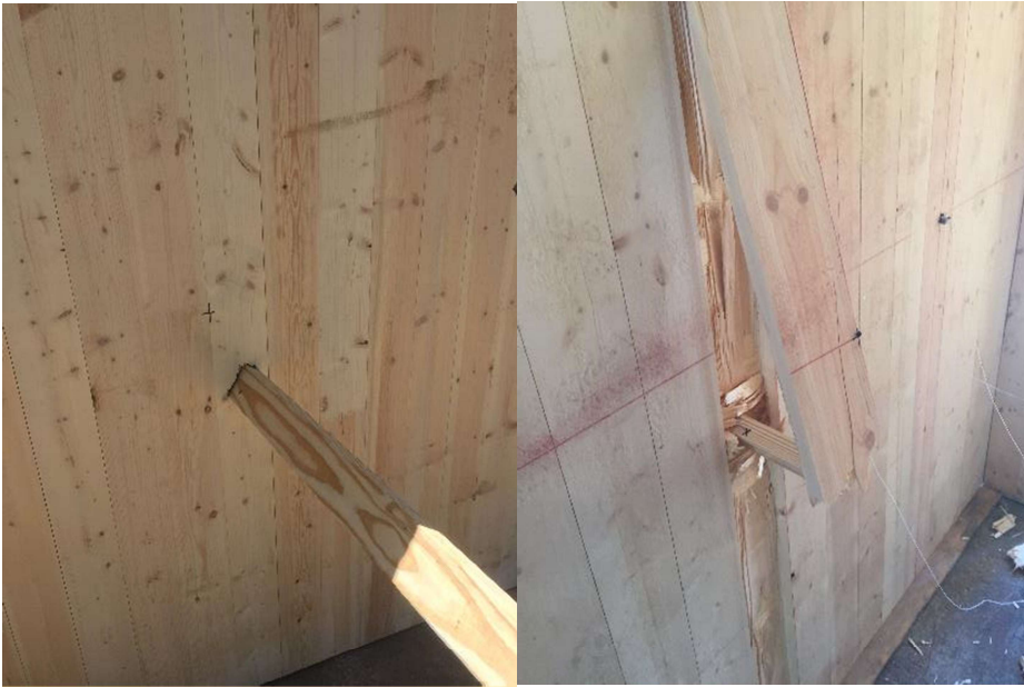
Figure A-10: Panel 4, weak-axis, strong-connection, center, 12-pound, 96.8 mph, failed – permanent deflection (front-left, back-right)
