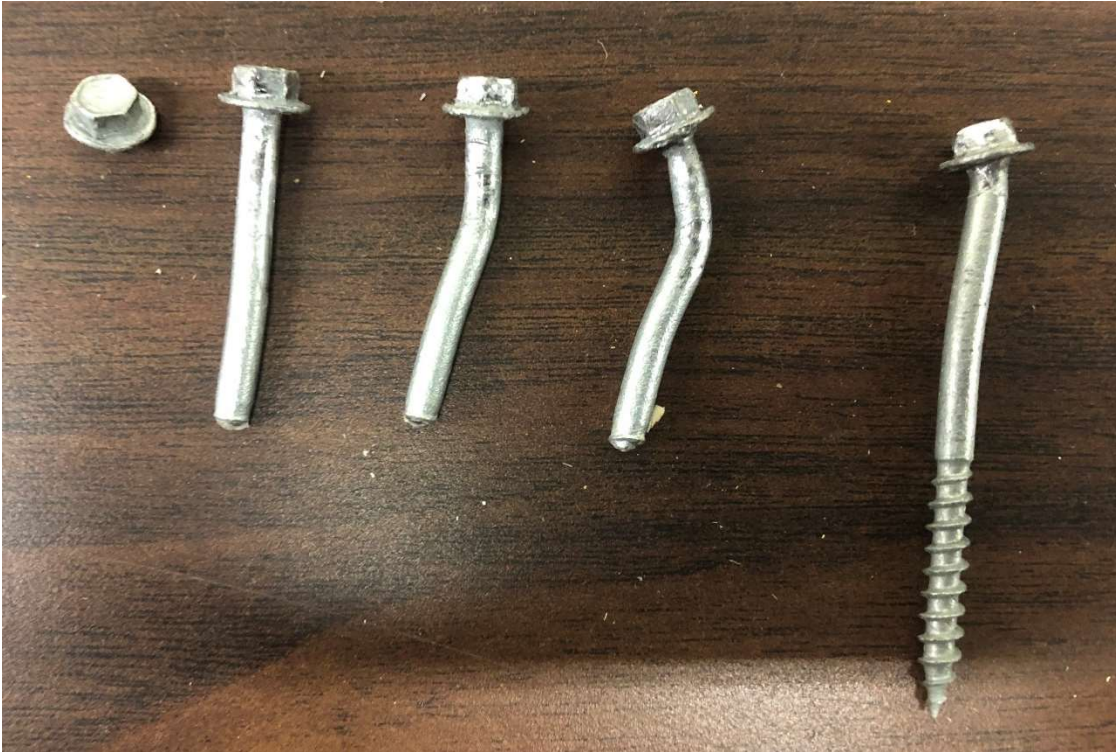
Figure 4.34: Deformation of SD10212 screws used in AE116 connection
