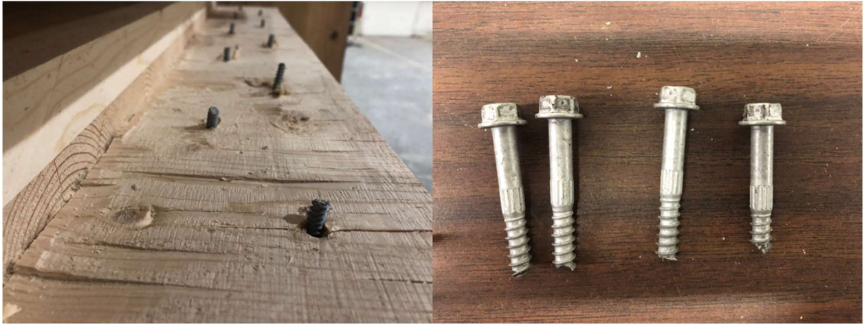
Figure 4.31: Failure of half-lap connection examined after wall assembly removal
