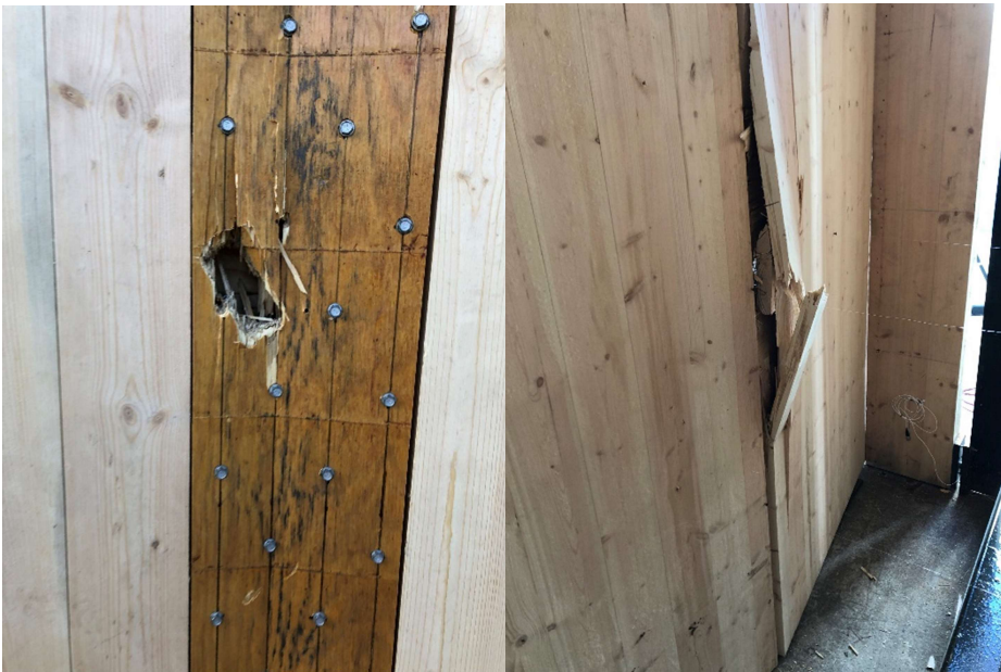
Figure A-45: Panel 17, weak-axis, surface-spline connection, center, 15-pound, 76.3 mph, failed – permanent deflection (front-left, back-right)
