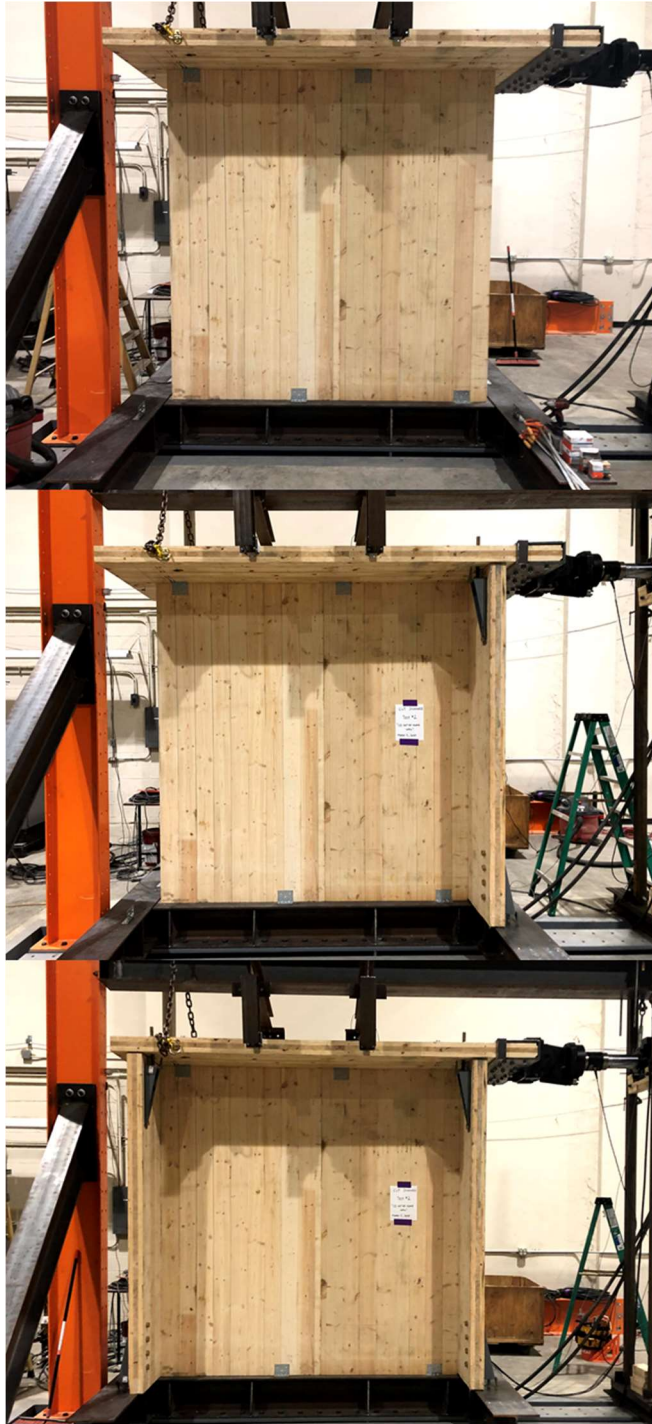
Figure 4.17: Progression of stiffness tests: in-plane only, one out-of-plane wall, two out-of-plane walls (top to bottom)
