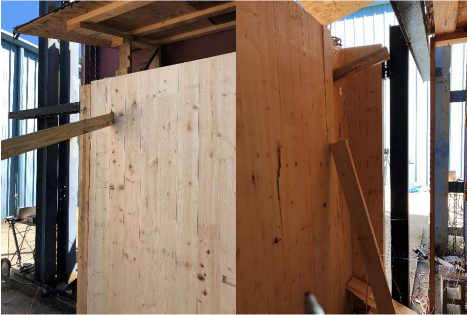
Figure A-42: Panel 14, weak-axis, weak-connection, corner, 9-pound, 89.5 mph, failed – perforation/dislodgement (front-left, back-right)
