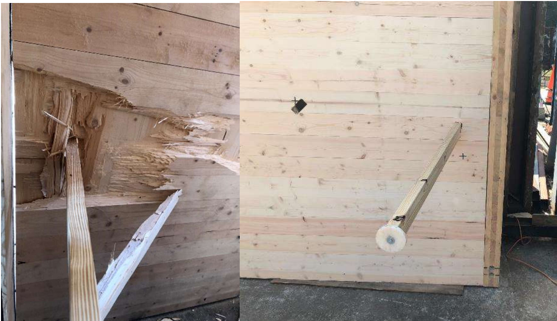
Figure A-29: Panel 10, strong-axis, weak-connection, edge, 15-pound, 112.8 mph, failed – perforation/dislodgement (back-left, front-right)
