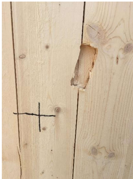
Figure A-18: Panel 6, weak-axis, strong-connection, corner, 12-pound, 69.7 mph, passed (front of panel)
