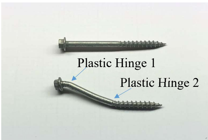
Figure 4.3: Deformed shape of screw tested monotonically in shear
