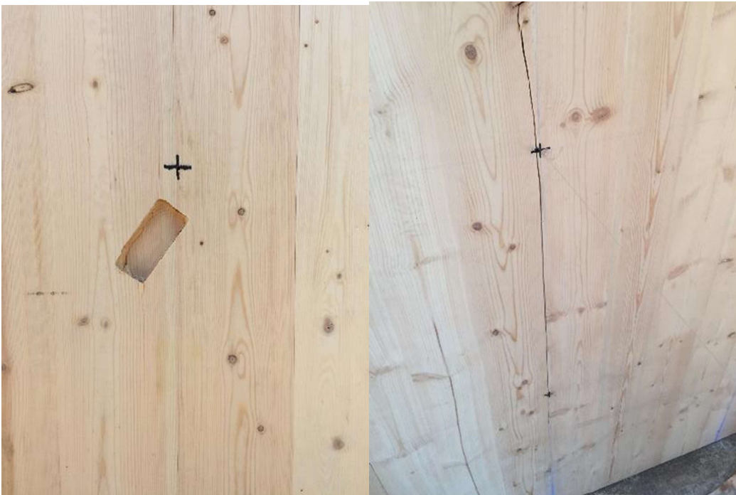
Figure A-13: Panel 5, weak-axis, strong-connection, center, 15-pound, 87.9 mph, passed (front-left, back-right)
