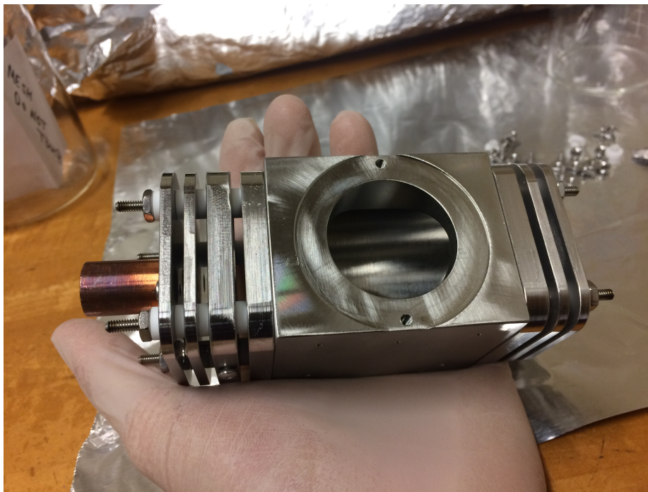
Figure 2.18 A photograph of the assembled FGC body. The order and purpose of each component mimics those of the MGC in Fig. 2.1.
