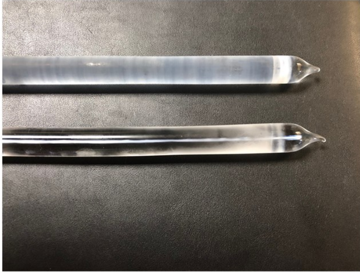
Figure 4.10: Reduction of devitrification in the core region from initial preforms (lower) to final preforms (upper).
