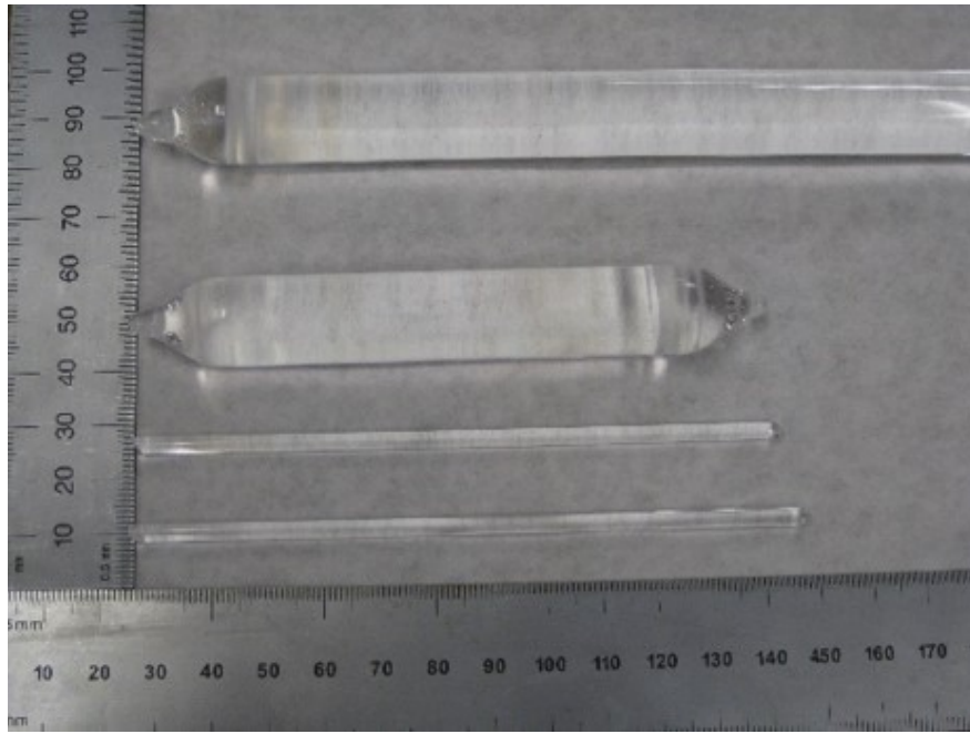
Fig 2.8. Starting preforms prior to grinding (top), shortened section (mid) and preform after clad removal and surface polish(bottom)
