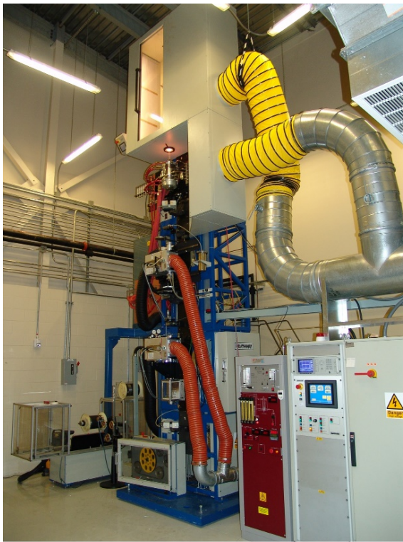
Figure 1.3: Clemson draw tower and typical tower layout [18]
