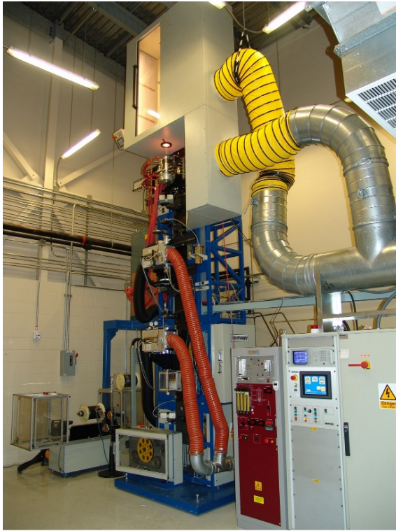
Figure 2.13: Clemson draw tower and typical tower layout [15]
