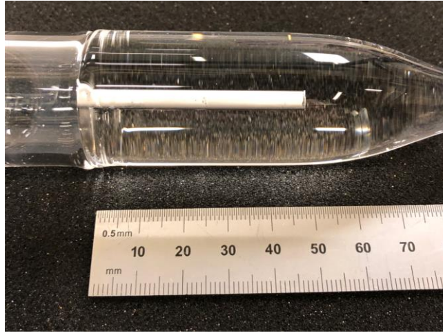
Figure III.13. Optical fiber preform with a calcium oxide coating the inner capillary. A silicon rod is within the capillary, but unable to be seen due to the opacity of the CaO coating.
