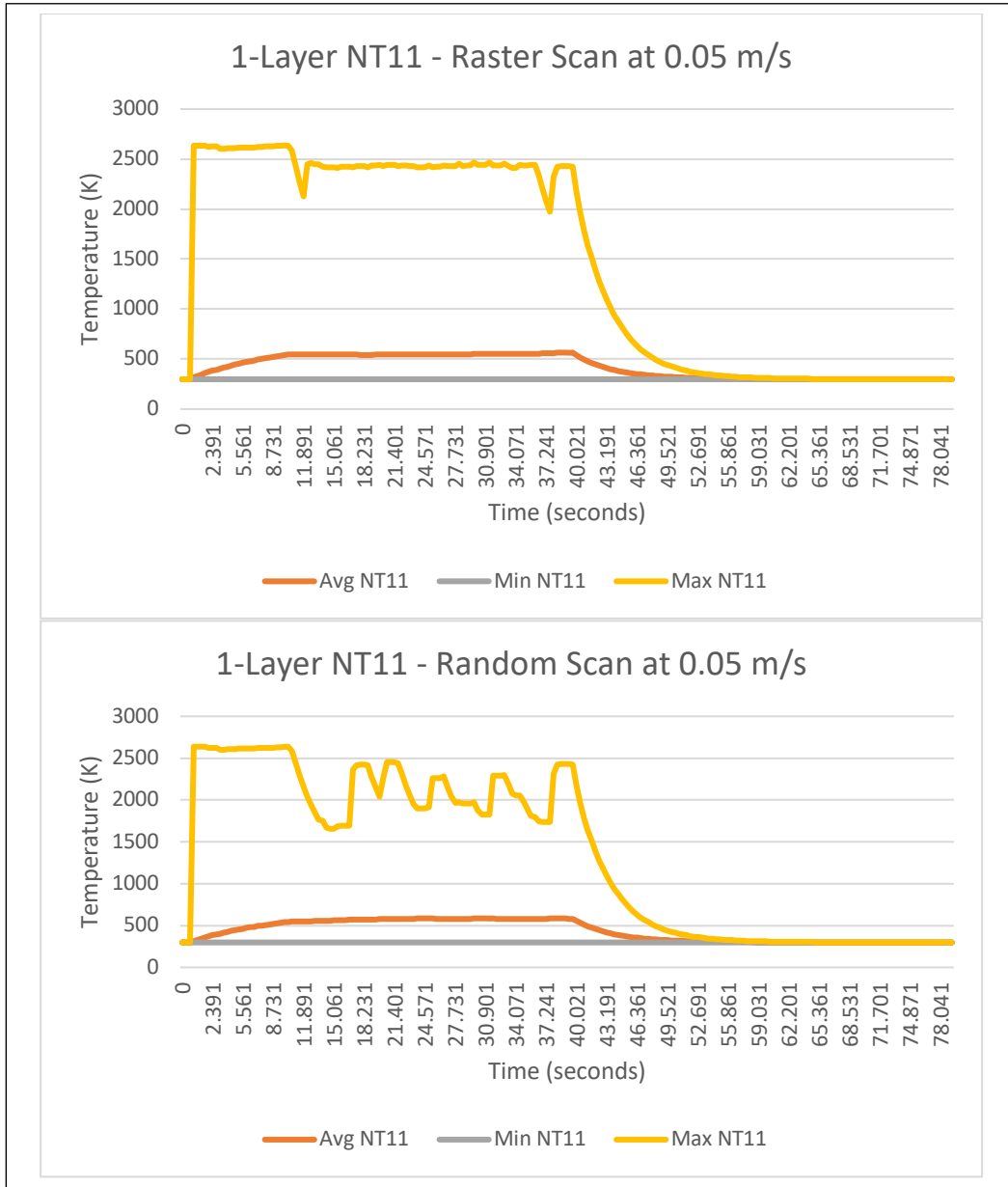
Figure 3. 15 NT11 Results for 1-Layer Random and Raster Scan at original parameters at Scan Speed = 0.05m/s
