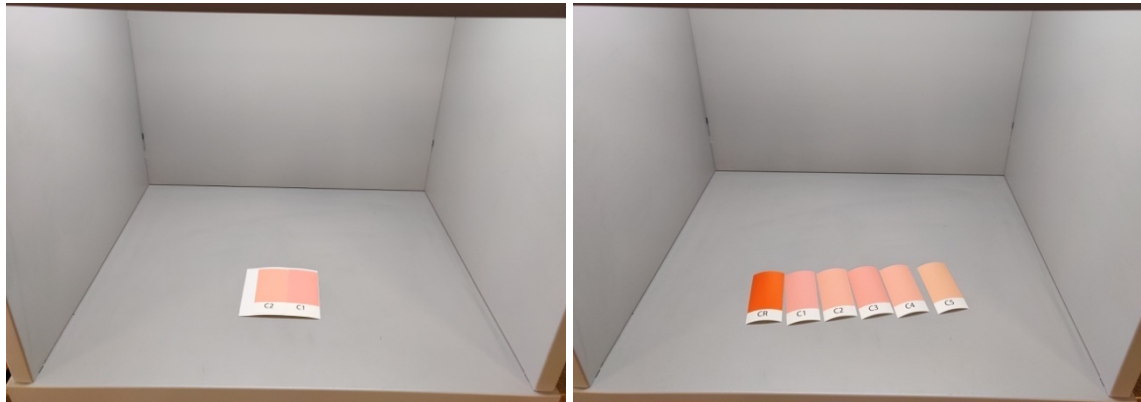
Fig. 4.4. Visual study setup – Pairwise comparison (left) and ranking (right) samples
