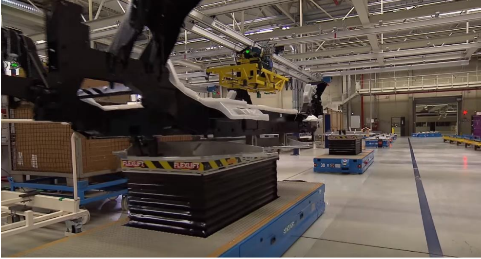
Figure 3: AGV moves chassis throughout factory (Physical: 6, Cognitive: 7)
