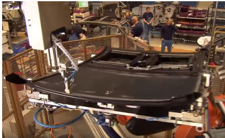
Figure 2.3. Machine Applies Adhesive to Roof
