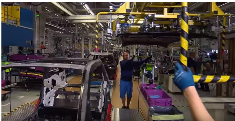
Figure 2.4. Lift Assist to Install Roof
