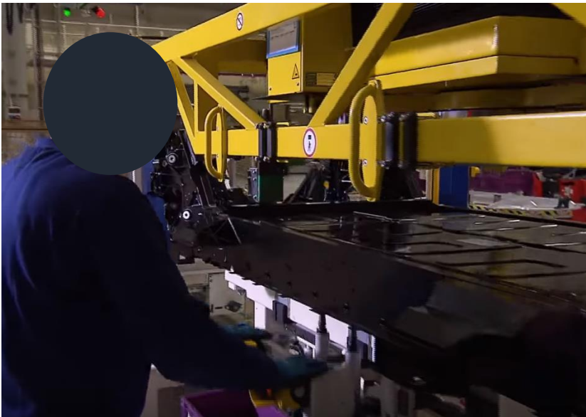
Figure 2: Operator moves drill so machine can install screws (Physical: 5, Cognitive: 3)
