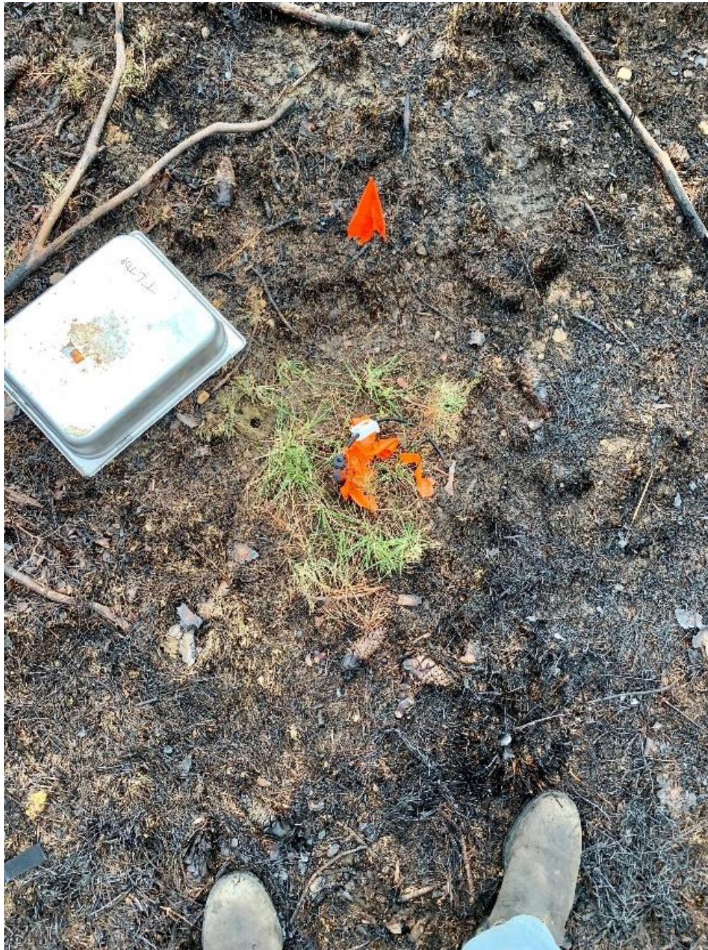
Figure 2.4: In-ground lysimeter installed post-fire with protective cover. Fuel consumption was representative of a low severity burn and soil heating was minimal as demonstrated by the effectiveness of the metal protective cover.
