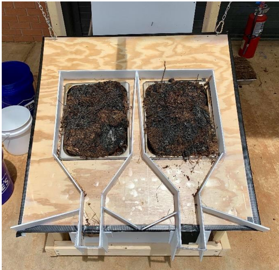
Figure 3.2: RFS sample mount with two Low-severity treatment Pine litter samples. Guard rails prevent runoff loss and a cover was placed over collection buckets to prevent sample saturation.
