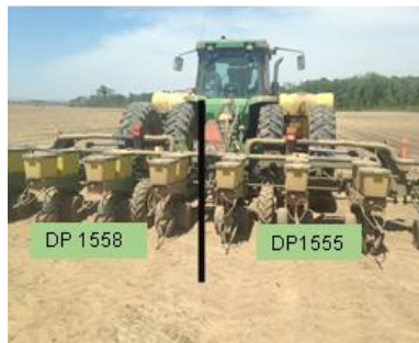
Figure 3-2. Commercial planter used to plant alternating 12-row strips across the entire study area in year one. Planter rows 1-6 were filled with DP 1558 and rows 7-12 were filled with DP 1555. Planting was done in sequential passes to achieve 12-row (15m) wide plots.
