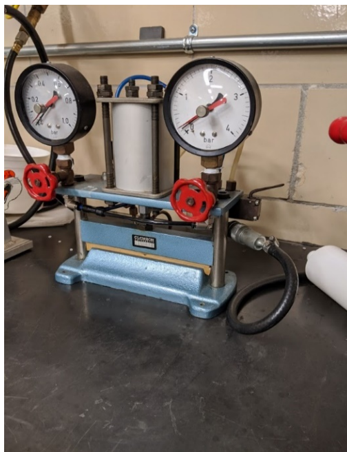
Figure 3.4.4: MECMAN series 1100 seal strength burst testing device
