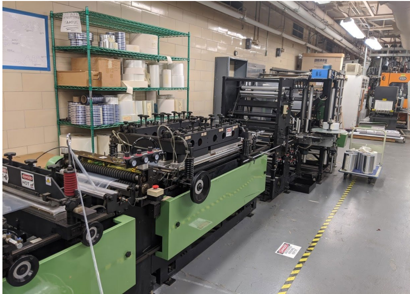
Figure 3.4.2: FSD-600SZ three side seal stand-up pouch machine – output end of machine
