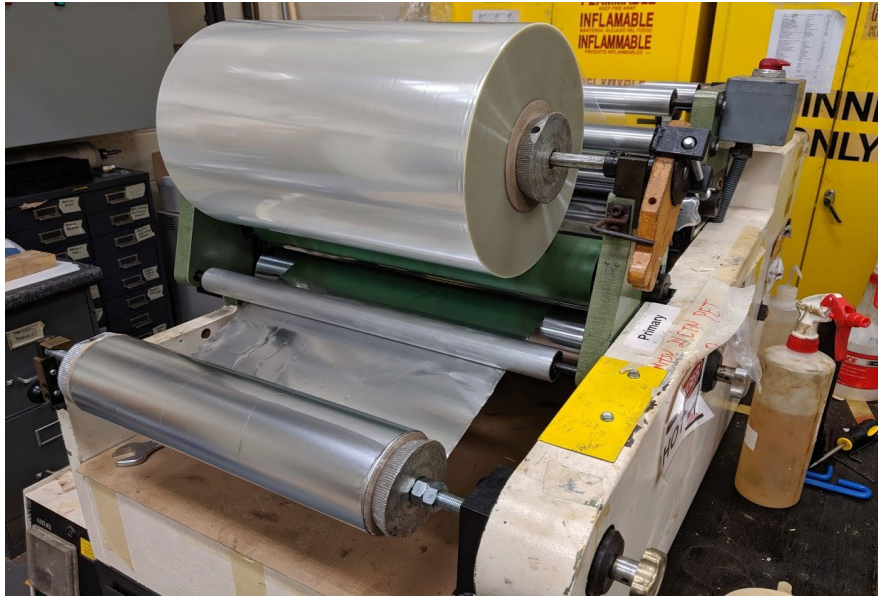
Figure 3.3.3: Polytype LTD. (Fribourg, Switzerland) series number 612'0614 Solvent-free lamination machine
