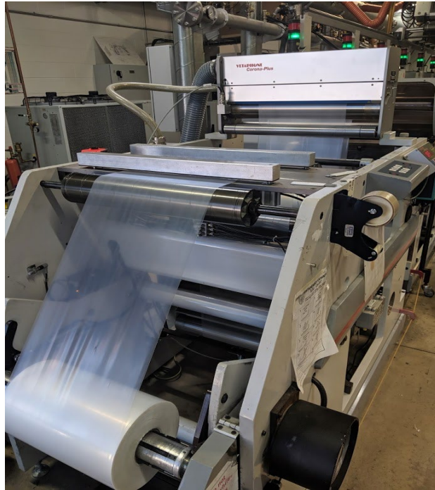
Figure 3.3.2: Vetaphone Corona-Plus type TF-415 corona treater installed on a Varyflex Omet VF 530F1 printing machine
