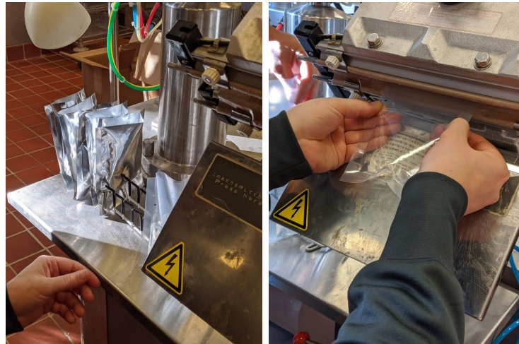
Figures 3.4.5: Set-up for sealing pouches 3.4.6: Sealing of pouches
