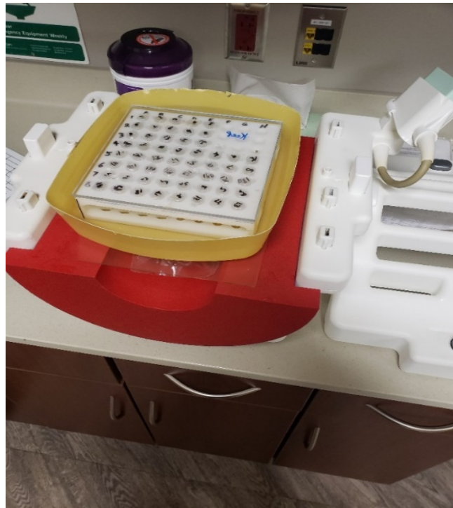
Figure 2.12) Image of experimental set up with the sample holder inside a head space coil a bucket filled with ProHance water surrounding the samples
