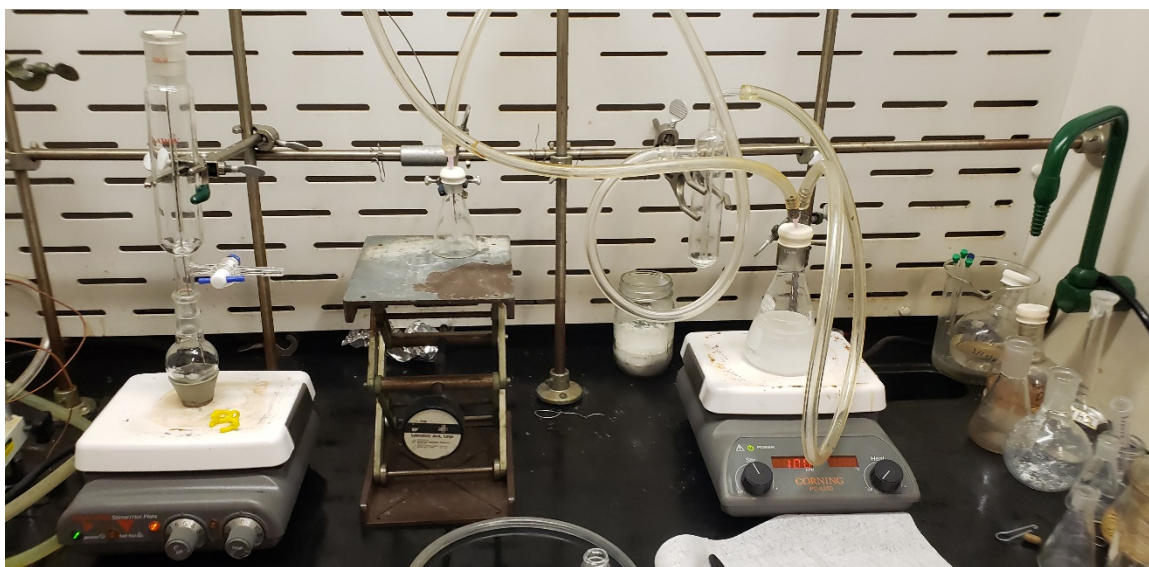
Appendix A.2- Set up of reaction for hydrogenation of n-BAPTA with hydrogen production reaction on the right and bubbling into reaction vessel on the left
