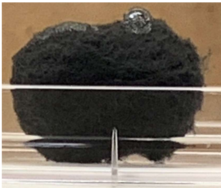
Figure 2.9: Image of pyrolyzed cotton ball with a drop of water supported on the surface due to the hydrophobic interaction between the pyrolyzed cotton ball fibers and the water droplet.
